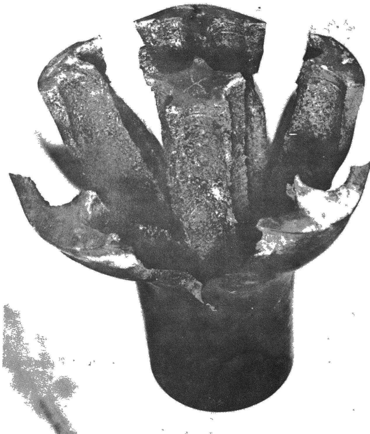
Fig. II-26. Cerium Metal Loaded Five-Hole Impact Cap Design
