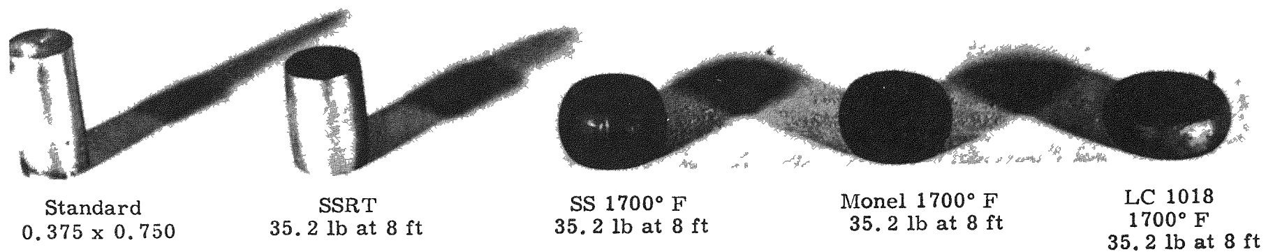
Fig. V-9. Impact Test Results on Different Materials at 1700° F and Room Temperature
