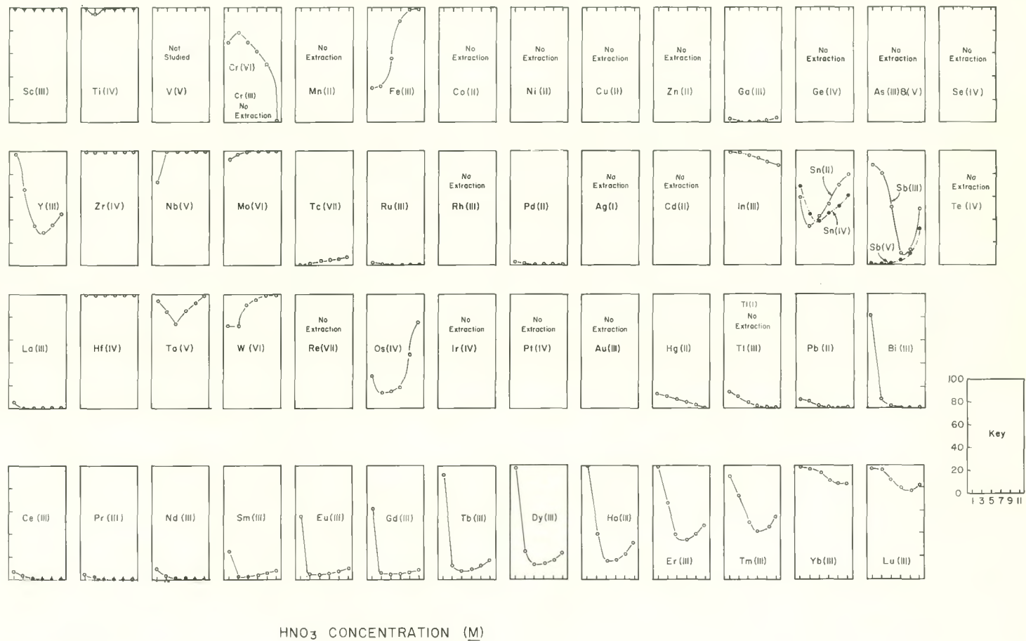
Figure 20. Extraction curves for bis(2-ethylhexyl) orthophosphoric acid as a function of nitric acid concentration.
