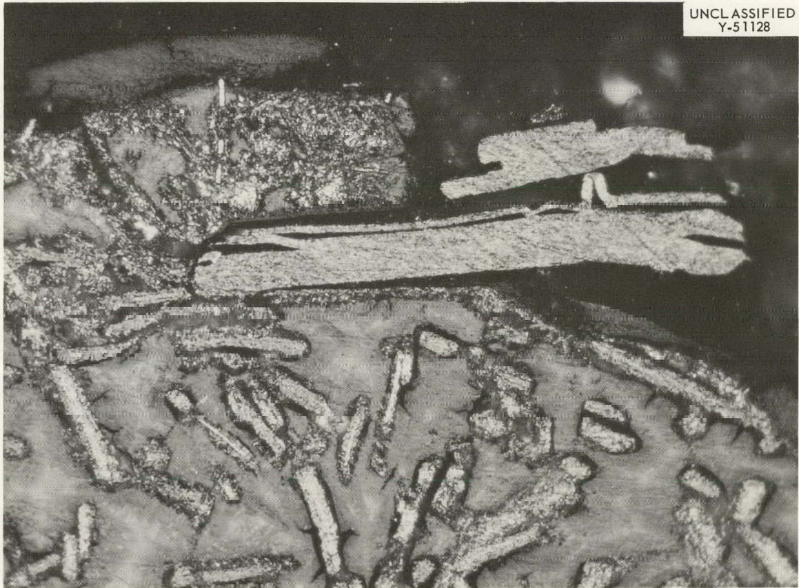
Fig. 6. Photomicrograph of Residue from (U,Th)C 2 Particles after Chlorine Treatment. 1000X.
