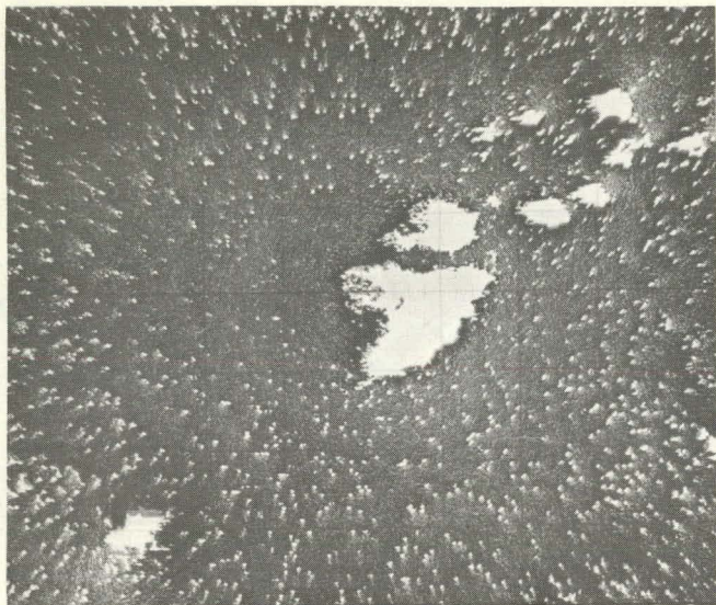
FIGURE 47. The aluminum- K_{\alpha} microprobe raster scan of the area in Figure 46. The aluminum count is 100,060 counts per 60 seconds in the inclusion area as compared to 117 counts per 60 seconds background and 293,235 from an aluminum standard. (Magnification 300X).
