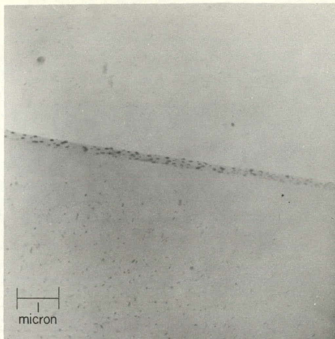
FIGURE 26. Grain-boundary and matrix precipitates in a beryllium sample brine-quenched from 1000°C and aged to 780°C for five minutes. In contrast to Figure 25, matrix precipitates are definitely in evidence.
