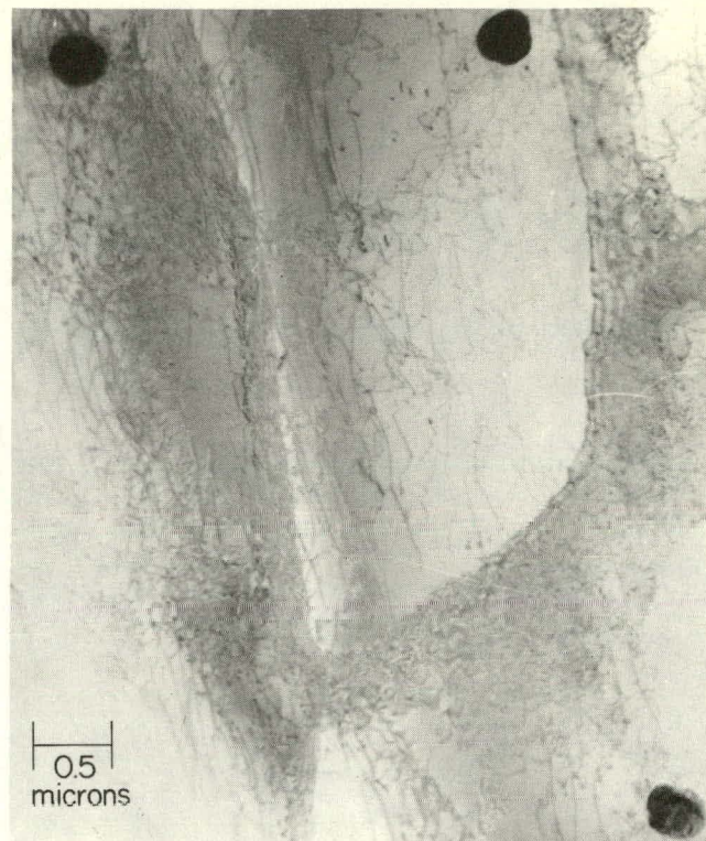
FIGURE 6. Precipitates (type \text{AlFeBe}_4 ) in the as-rolled beryllium foil.
