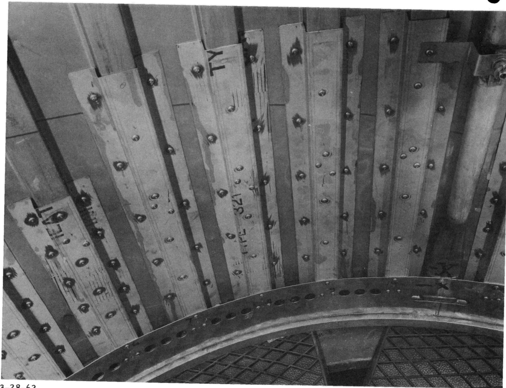
Figure 10. Repair of Damaged Corrugations
