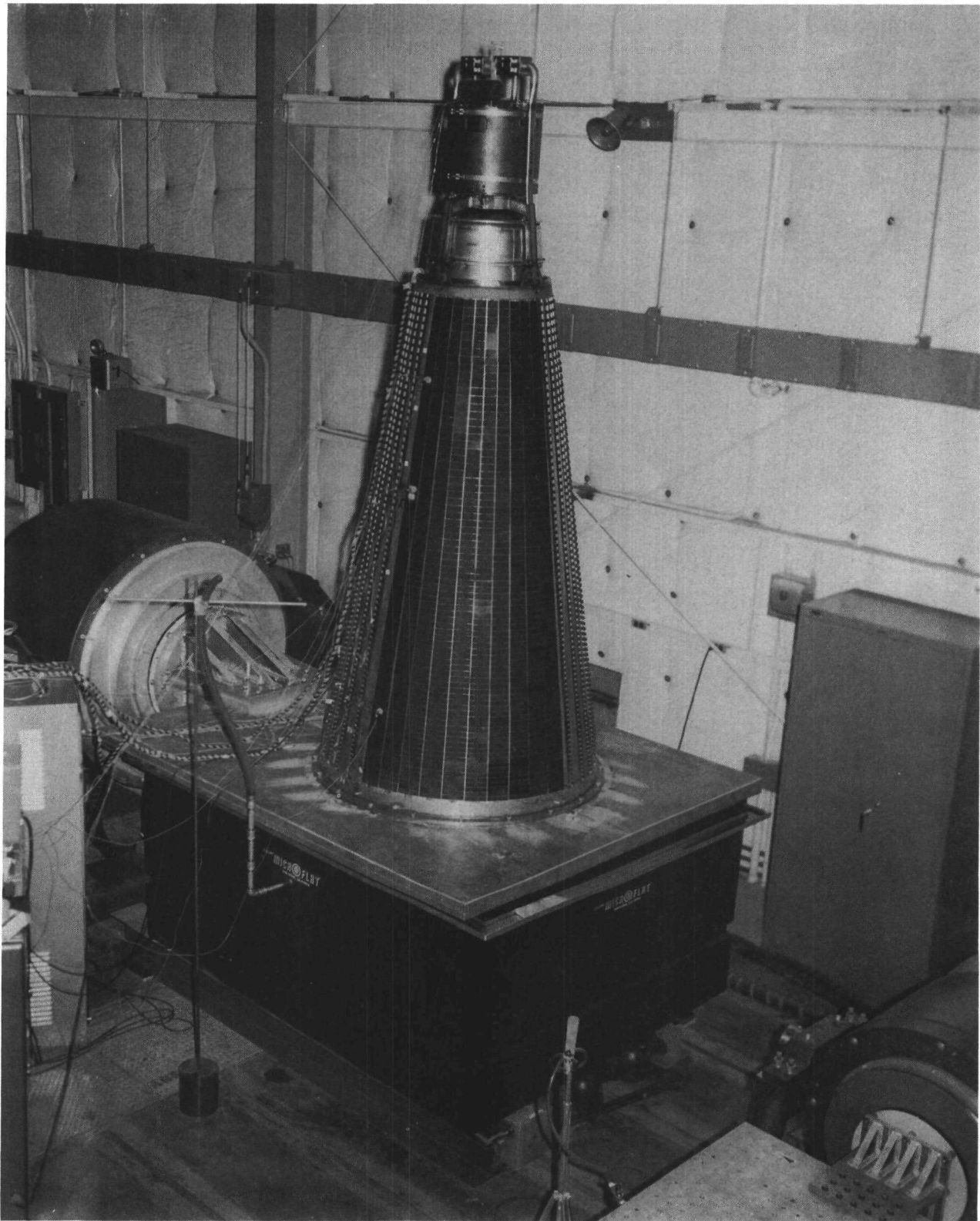
Figure 5. S10A-PSM-1 Vehicle Mounted on the Slip Table for Lateral Excitation
