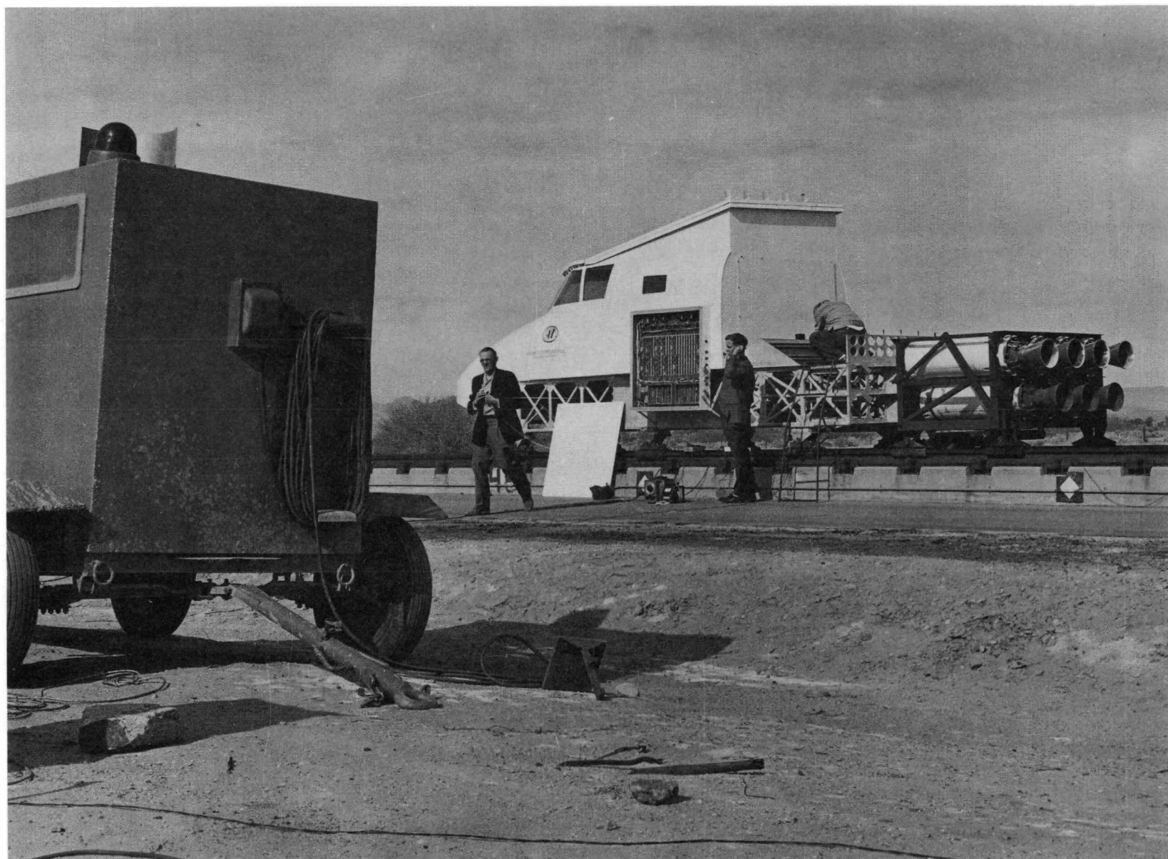
Figure 32. Rocket Sled Utilized for PSM-1 Acceleration Studies
