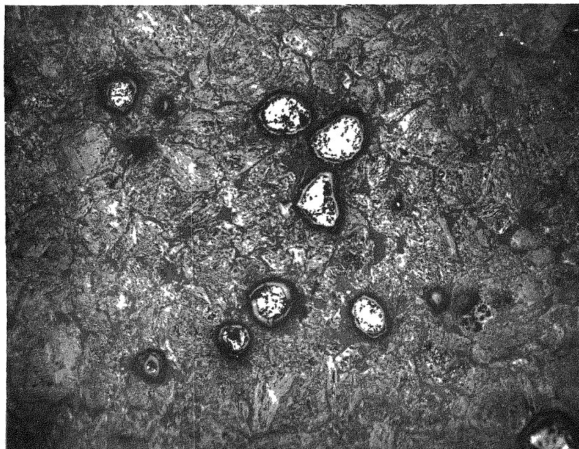
Fig. 2-6. Graphite- \text{Al}_2\text{O}_3 Specimen Type 1, as fabricated (50X).
