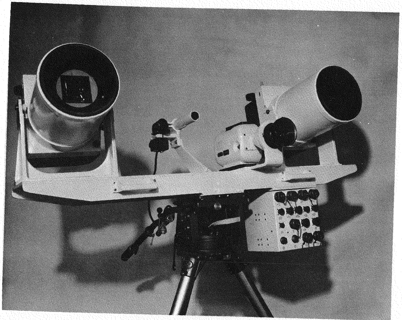
Figure 11. Handtracked Streak Spectrographs. By using two streak spectrographs per mount, a larger field of view is covered.
