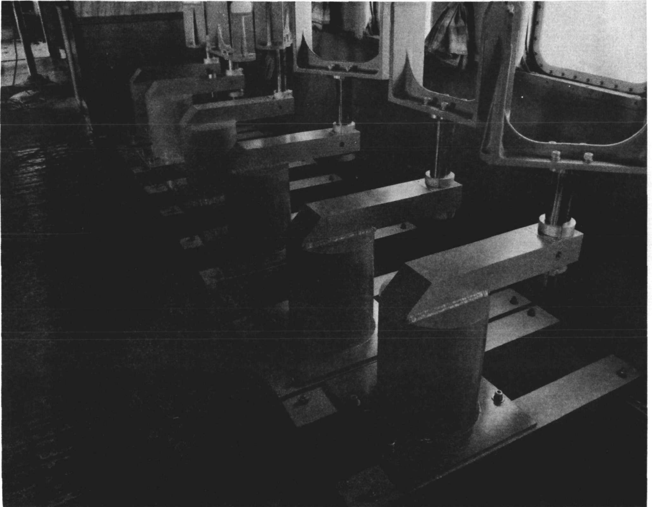
Figure 15. Typical Camera Mount Arrangement in Aircraft. Bolting to the seat rails allows longitudinal adjustment. Transverse, vertical, and 2 degrees of rotational adjustments are also provided.
