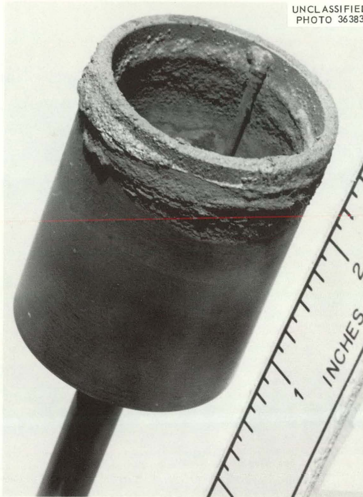
Fig. 2.11. INOR-8 Solder Freeze-Valve Cap After Testing.
