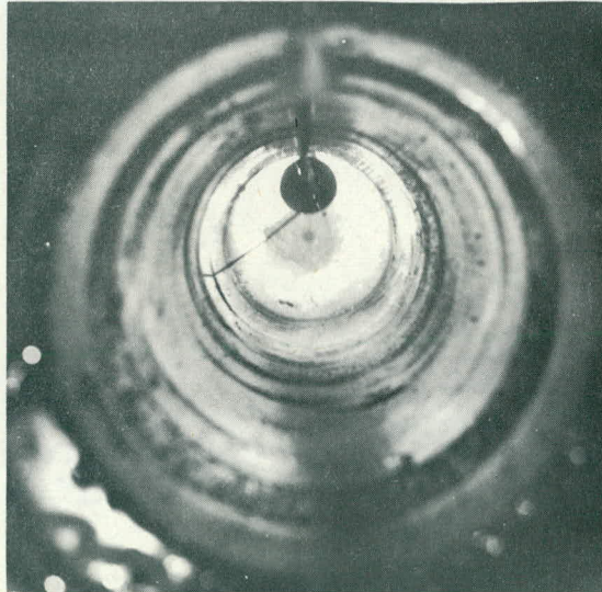
(4) UNDERWATER LAMP (1000 WATT) FACE-DOWN THROUGH 10 FEET OF WATER (5 FLUSHES WITH WATER TEMPERATURE 70 °F.), RUN No. 5
