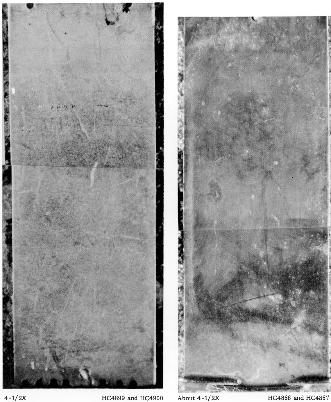
FIGURE 13. APPEARANCE OF TWO ADDITIONAL SPECIMENS AFTER IRRADIATION
