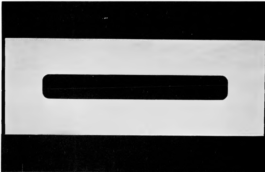
FIGURE 2. SM-2 REFERENCE TYPE 347 STAINLESS STEEL PICTURE FRAME USED FOR FABRICATING IRRADIATION SPECIMENS
