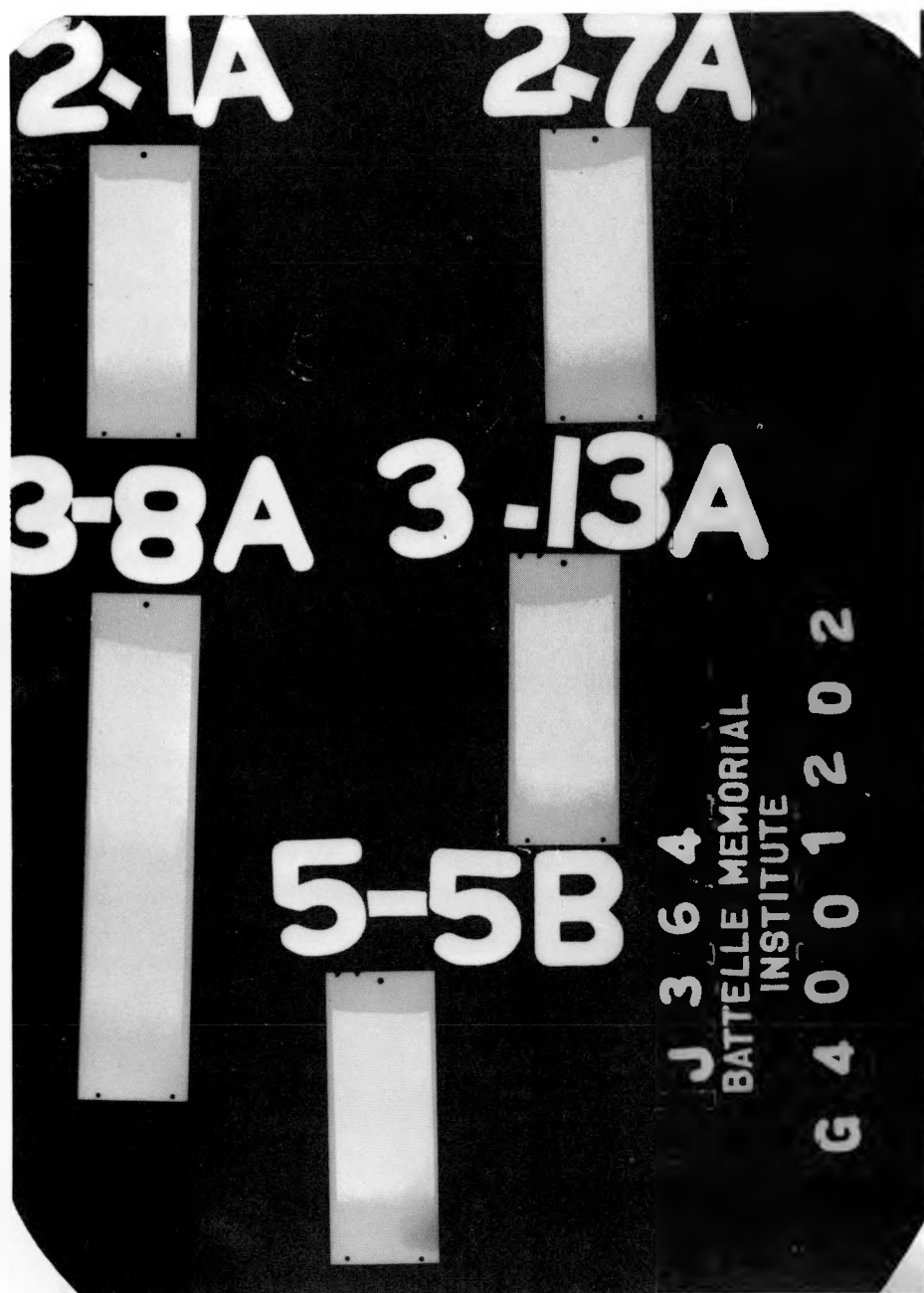
FIGURE 9. PREIRRADIATION RADIOGRAPH OF A CAPSULE LOADING OF SM-2 IRRADIATION SPECIMENS
