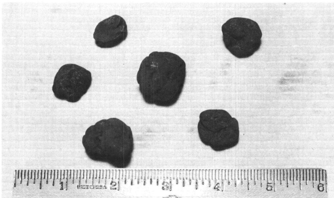
FIGURE 13 URANIUM ISOLATED FROM MAGNESIUM-RICH SYSTEMS BY RETORTING
