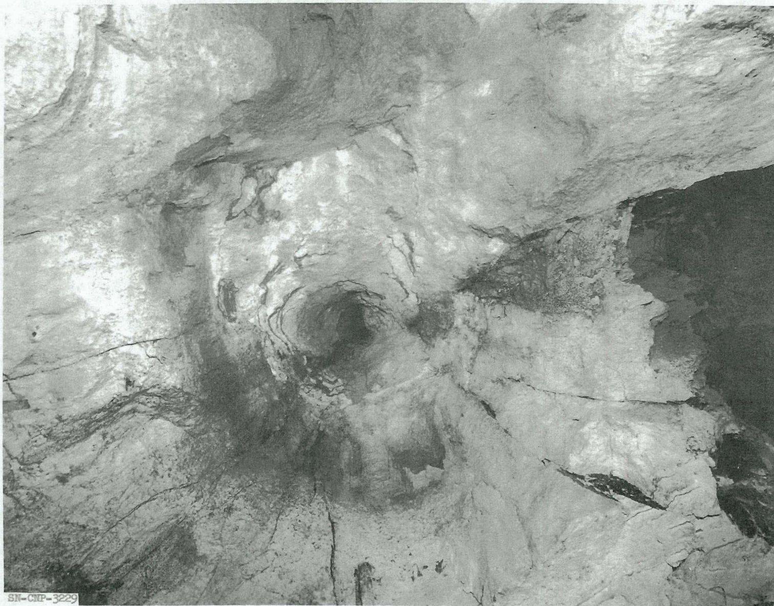
Fig. 7. View of top of Hobo Shot 11 cavity, explosive loading hole in center, showing initial radial character of fractures. Bottom of picture to east; right to south.
