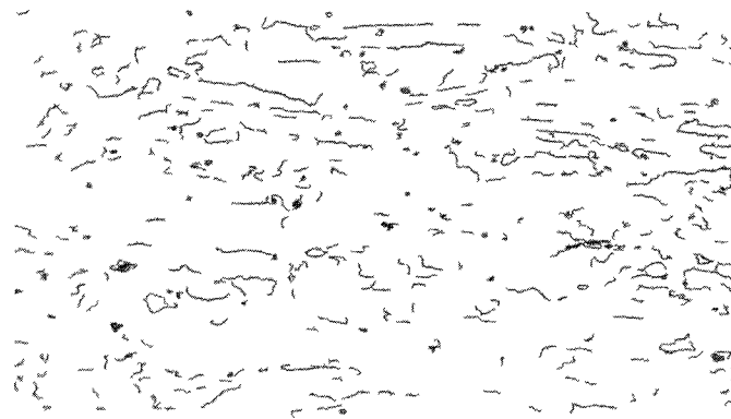
FIGURE 39. NIOBIUM-10 w/o URANIUM ALLOY COLD WORKED TO 90 PER CENT REDUCTION IN THICKNESS AND ANNEALED 1 HR AT 2400 F
