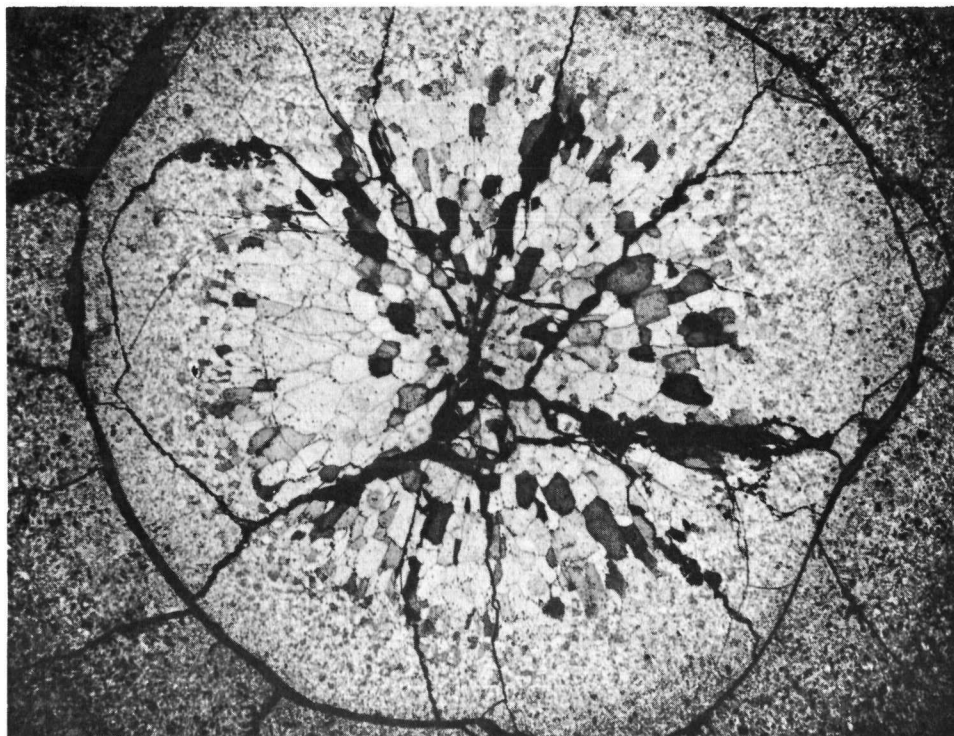
Fig. 10 Equi-axed grain growth in UO_2 from bundle P.
