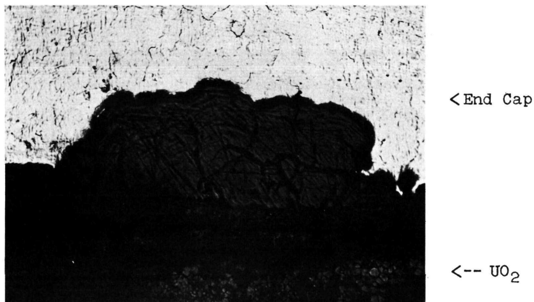
Fig. 31 (b) Localized corrosion at \text{UO}_2 /Zircaloy interface. Lower end cap.
