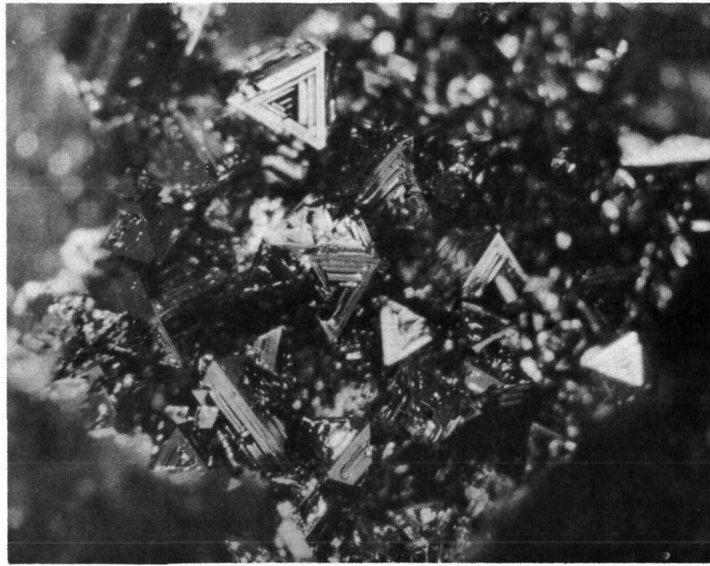
Fig. 13 Vapour deposit found in central void of element P-2.
