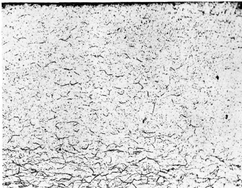
Fig. 21 \text{ZrH}_2 precipitation in sheath of element K-2 showing higher concentration at outer surface.
