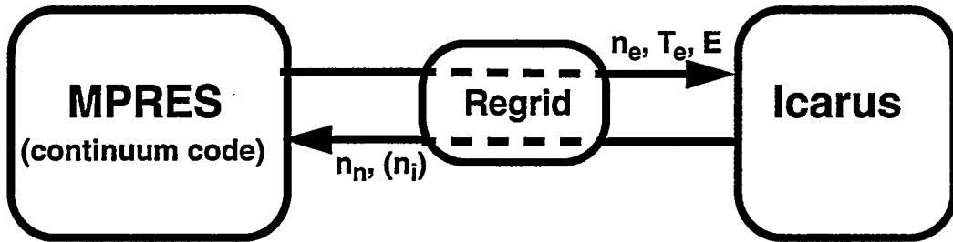
Two different strategies that can be used to couple MPRES and Icarus; weak coupling, and strong coupling. The coupling strategy determines how much information is cycled between MPRES and Icarus during a Gemini simulation. Coupling strategies are defined below:
