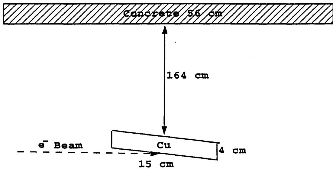
Figure 2. Geometry Used for PICa Simulation
