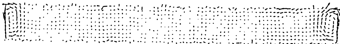
Fig. 3: Long-term average velocity field ( W/d = 100d , a = 0.5d , \Gamma = 10g , f = 7\text{Hz} ).
