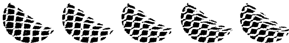
Figure 1. Grid-tag experiment of flowing mustard seeds at 18 rpm. The delays between tagging and imaging are 1, 10, 20, 50, and 100 ms, from left to right. The tagged cells translate and deform as a function of time.
