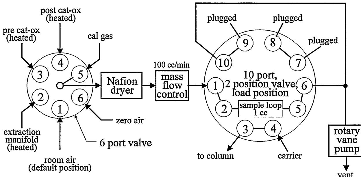
Because of the extremely high relative humidity of the samples, a Nafion™ membrane dryer is used for drying all samples upstream of the mass flow controller and sample loop. In the worst case design condition, the dryer is designed to reduce sample dew point to 0°C or lower. Although we have attempted by design to minimize the potential for condensation of water and or VOCs, we have no means for verifying that condensation does not occur.
