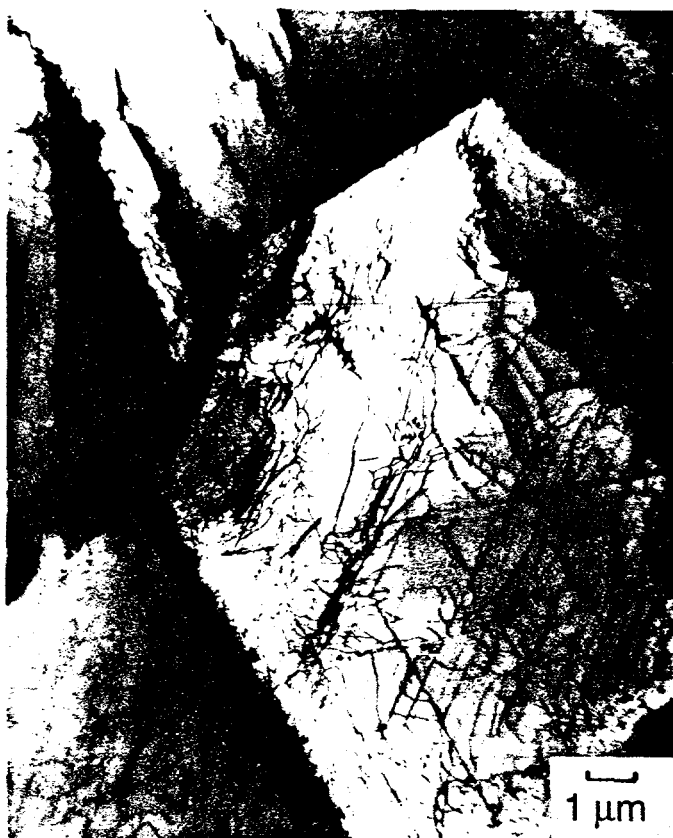
Fig. 10. Microstructure in sample taken from shoulder of a fatigue sample. Note absence of extensive dislocation structure.
