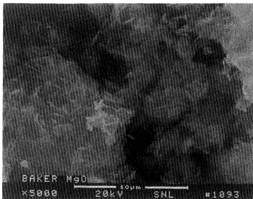
FIGURE 7. SEM Photomicrograph of Baker MgO After Calcining at 600°C/4 Hours
