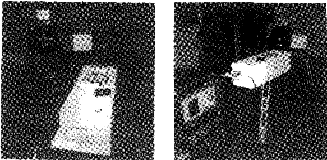
Figure A-10. Experimental Setup to Measure Horizontal (H-Plane) Time-Domain Pattern of Solid-Plate TEM Horn Antenna.
