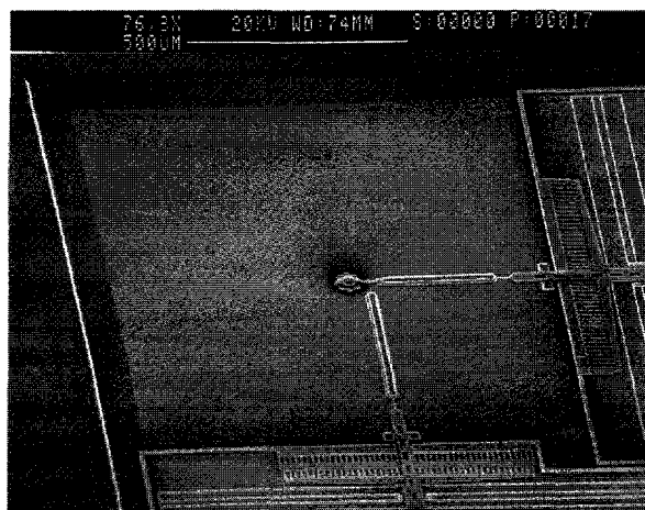
Figure 4. A three-level polysilicon structure (microengine) built in a trench. Here, the trench depth is approximately 12 \mu\text{m} .
