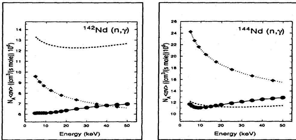
Figure 1. Astrophysical reactivities,  $N_A < \sigma v >$ , for  $^{142}\text{Nd}$  and  $^{144}\text{Nd}$ .  $\circ$  represent the ORELA data with an overall uncertainty of less than 6% for  $^{142}\text{Nd}$  and 3.5% for  $^{144}\text{Nd}$  respectively.  $\diamond$  are the experimental data from ref. 16, the dashed curve is the theoretical fit from ref. 17
