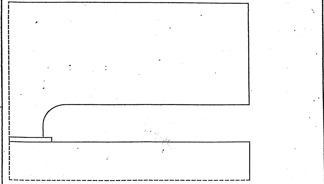
Figure 1. 2-D shape defined for the 118MHz cavity
