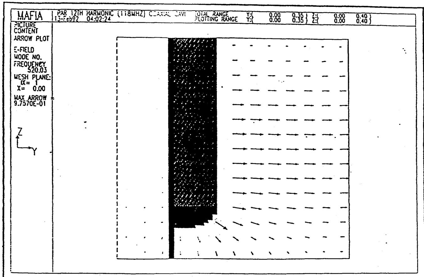
Figure 7. Electric field plot of the 118MHz cavity
