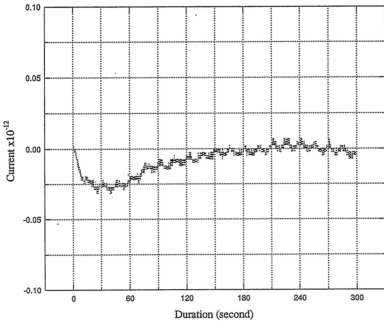
Figure 4. A printout from the data acquisition system used in conjunction with the Faraday cage. The result was obtained with a quartz sample (60 $\mu$ m)
