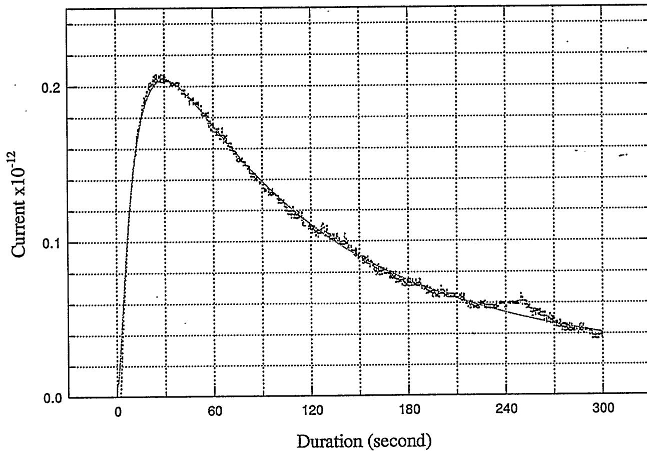
Figure 6. A printout from the data acquisition system used in conjunction with the Faraday cage. The result was obtained with a Pittsburgh No. 8 coal sample (-65 x 100 mesh)
