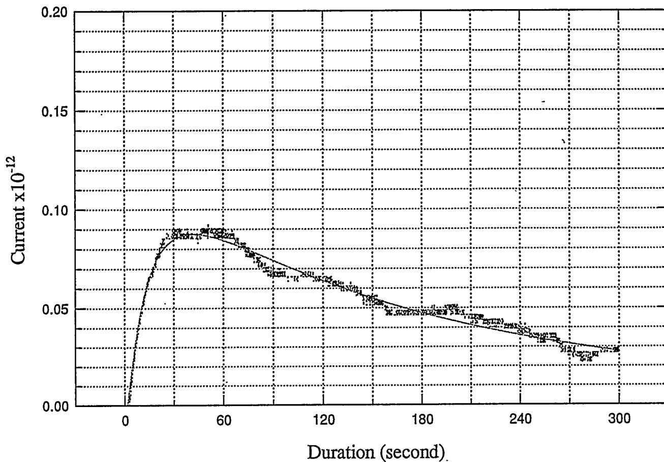
Figure 5. A printout from the data acquisition system used in conjunction with the Faraday cage. The result was obtained with a Pittsburgh No. 8 coal sample (+65 mesh)
