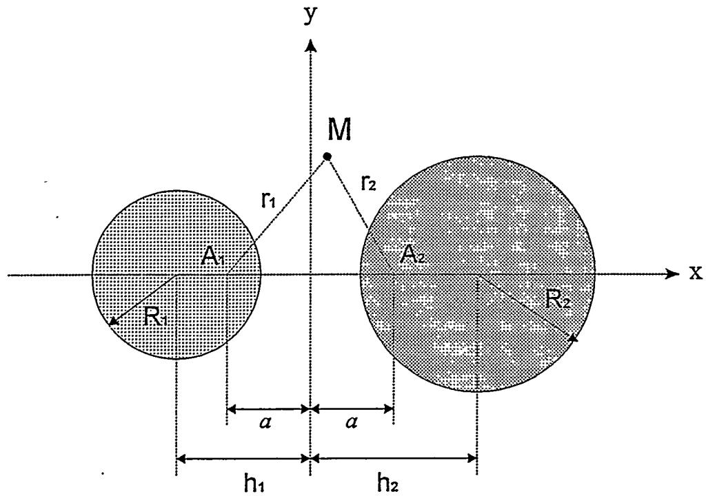
Figure 9. Calculation of the potential ( $\phi$ ) at point A in space in the non-uniform electric field created between cylindrical electrodes of radius  $R_1$  and  $R_2$ . The charges of the electrodes are represented by the point charge ( $\sigma$ ) at point  $A_1$  and  $A_2$
