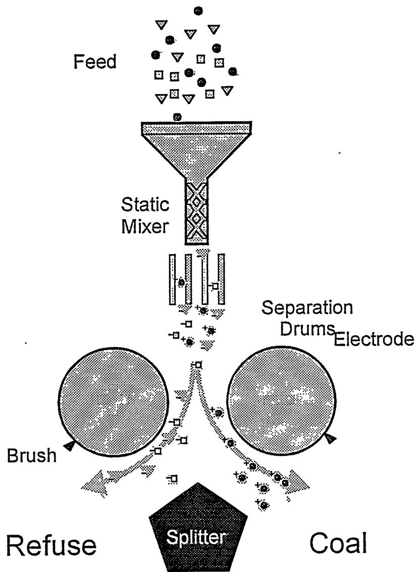
Figure 7. Schematic representation of the open-gradient triboelectrostatic separator used in the present work
