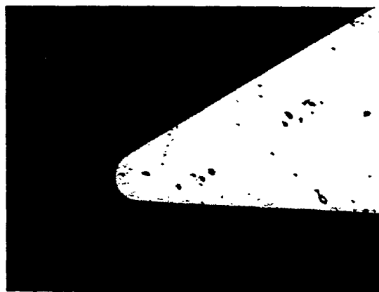
Diamond tool with a 25 \mu\text{m} radius tip
