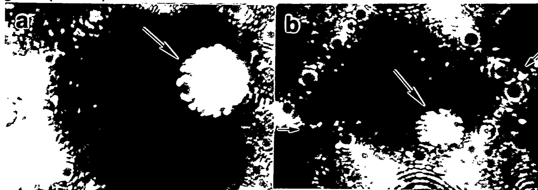
Fig. 6. Field ion micrographs of brightly-imaging Mo-rich precipitates that were detected in the matrix (Fig. 6a) and at grain boundaries (Fig. 6b) in the two alloys.
