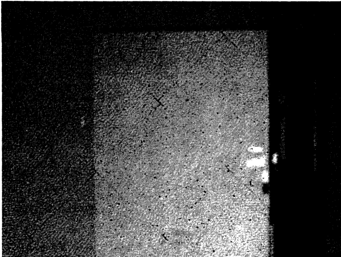
Figure 7. Diamond pattern of systematic error from the fiber optic faceplate is clear in this enhanced view of a portion of reflectance image taken from Station 10.
