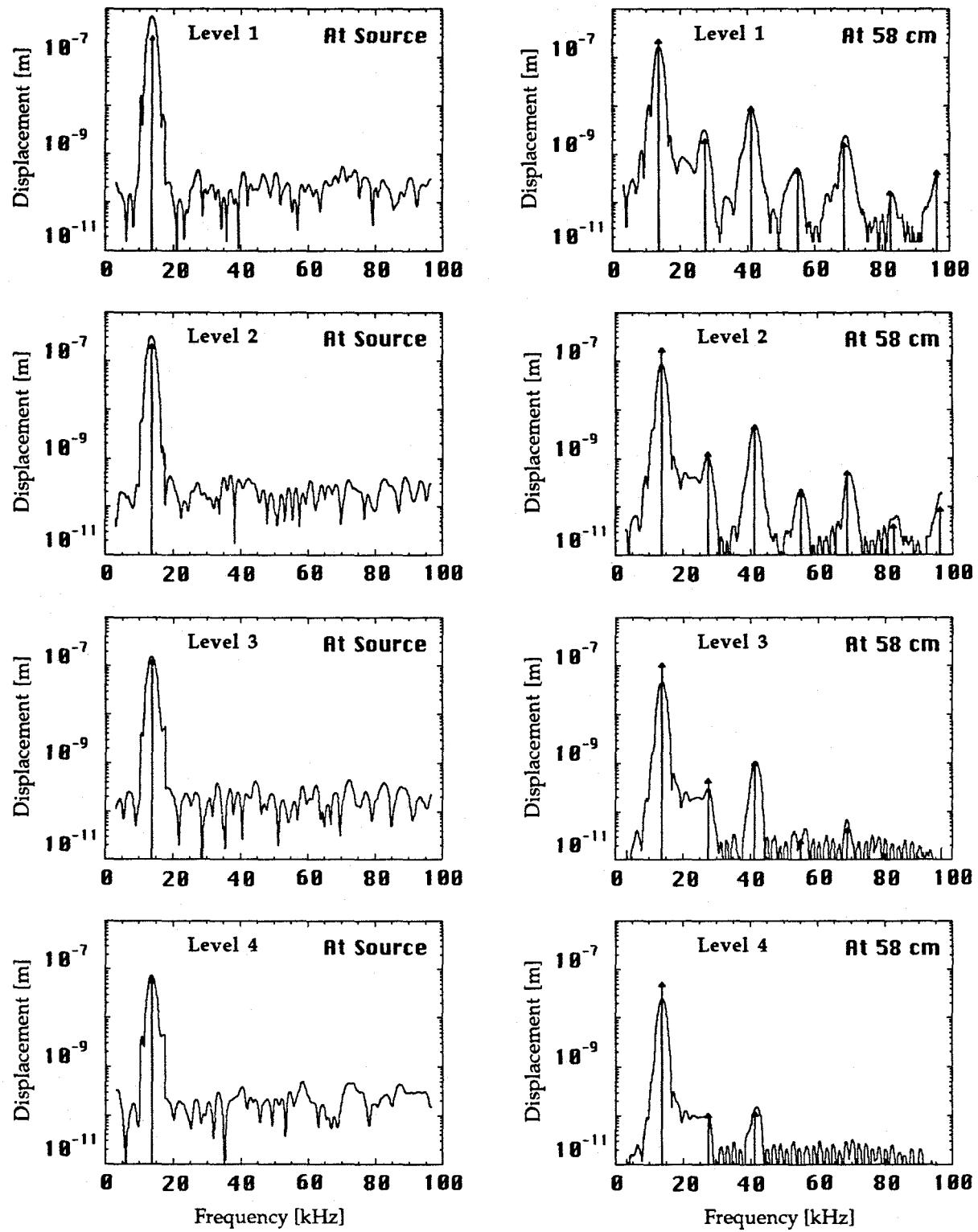
**Figure 1:** Experimental source and receiver (at 58 cm) spectra for a 13.75-kHz drive at 4 intensity levels (continuous lines) in a Berea sandstone bar and corresponding theoretical simulations using a 1D perturbation method (solid triangular-topped bars).
