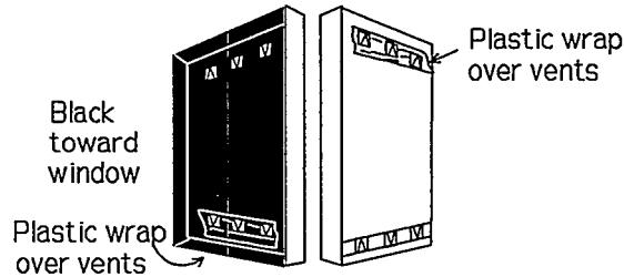
9. Cut enough plastic wrap to cover the vent holes and tape the plastic to the outside (black side) of the bottom vent holes and to the inside (string side) of the top vent holes.
