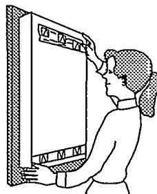
10. Slide the cardboard inside the window frame with the black side facing the window and the top vent holes up. (The plastic flaps should be hanging over the vent holes.) Tape the cardboard to the window frame with masking tape and leave an air space between the window and the cardboard.
