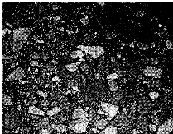
FIGURE 3. PBX 9501 HOT PRESSED TO 16% POROSITY, EPOXY-MOUNTED, POLISHED AND VIEWED BY PLM.
