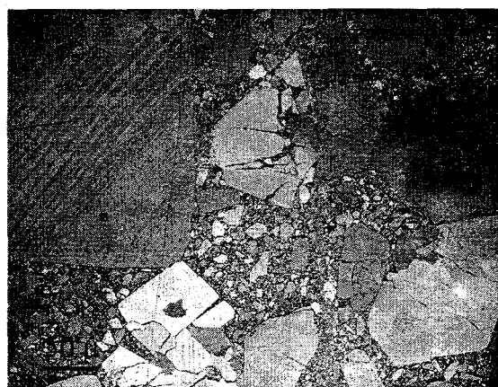
FIGURE 7. PRILL BOUNDARY IN PBX 9501 HOT PRESSED TO 7% POROSITY
