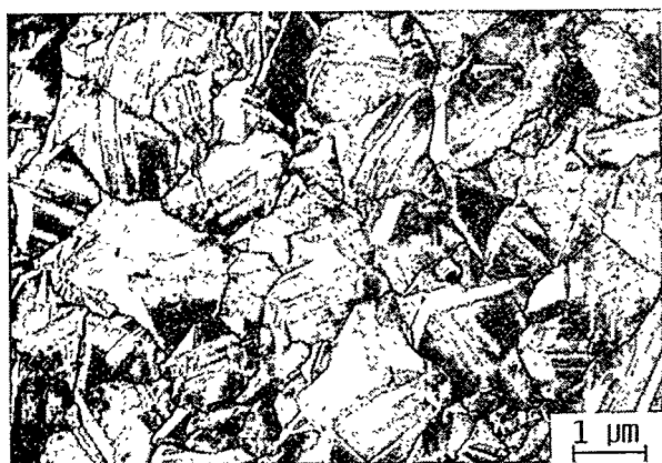
Fig. 17. Intergranular nature of the fracture surface during fracture-toughness testing of free-standing diamond films.
