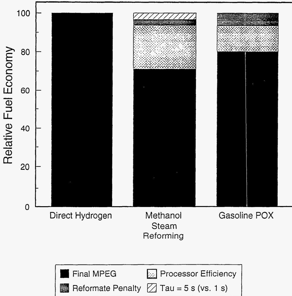
Fig. 11 Cost of Components in Alternative Fuel Cell Automobiles
