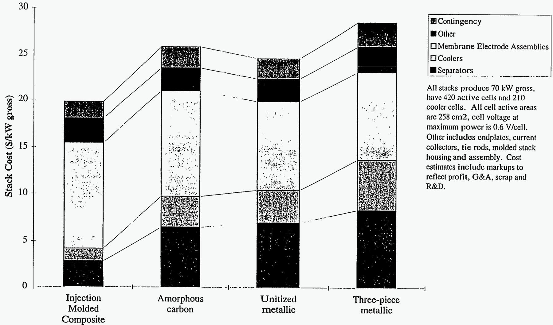
**Figure 7: PEM Fuel Cell Stack Cost vs. Stack Architecture**
