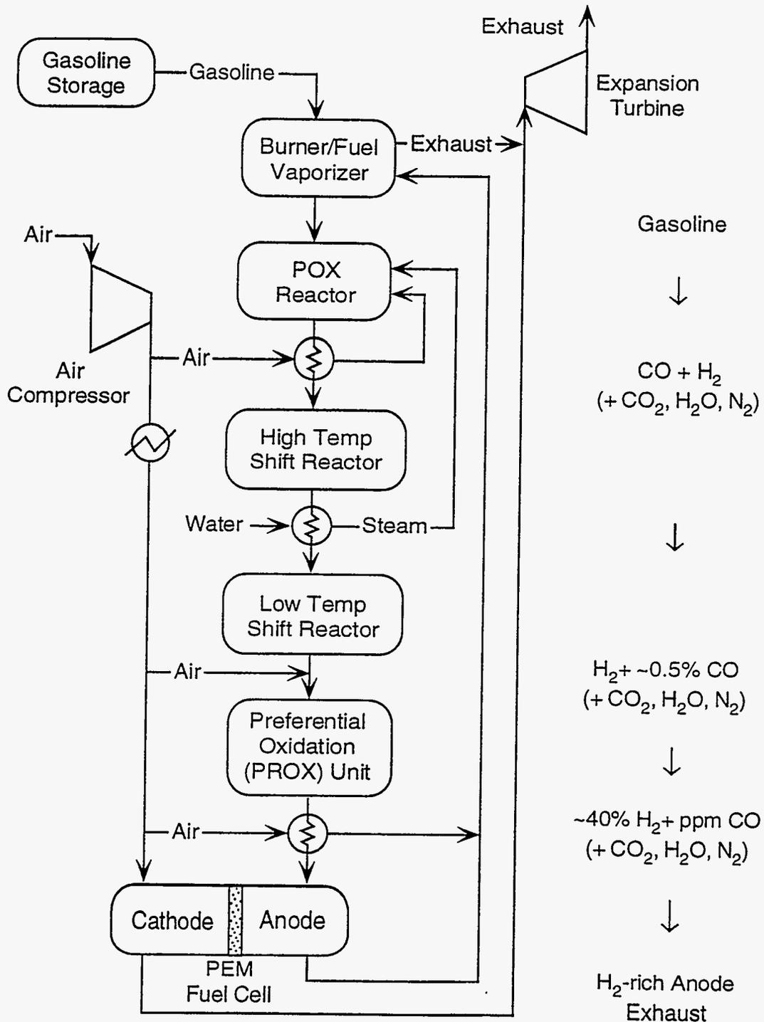
Figure 4. Schematic on-board gasoline partial oxidation (POX) reforming system.
