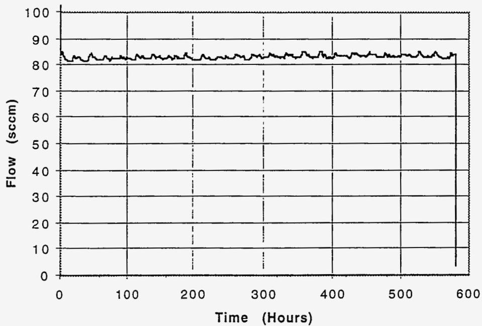
Figure 5. The performance of the membrane with 1,000Å of palladium on each side is slightly better than that with 5,000Å.
