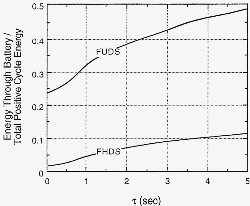
*Figure 7.* The fraction of the total positive cycle energy, for both the FUDS and FHDS driving cycles, that passes through the peaking device (e.g. battery), which acts as a buffer between the fuel processor/fuel cell system and the rapidly fluctuating demands of the driving cycle. Conditions: 1000 kg vehicle mass, 0.36 kWh battery, 1 sec characteristic time for battery recharging, 28.9 kW baseload power, 0.77 motor/controller efficiency.
