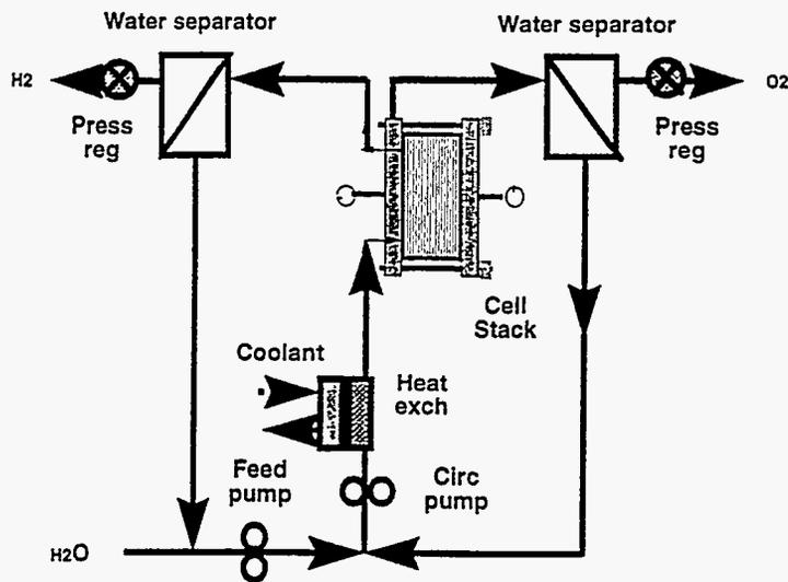
Figure 11 HOGEN Hydrogen Generator Physical layout
