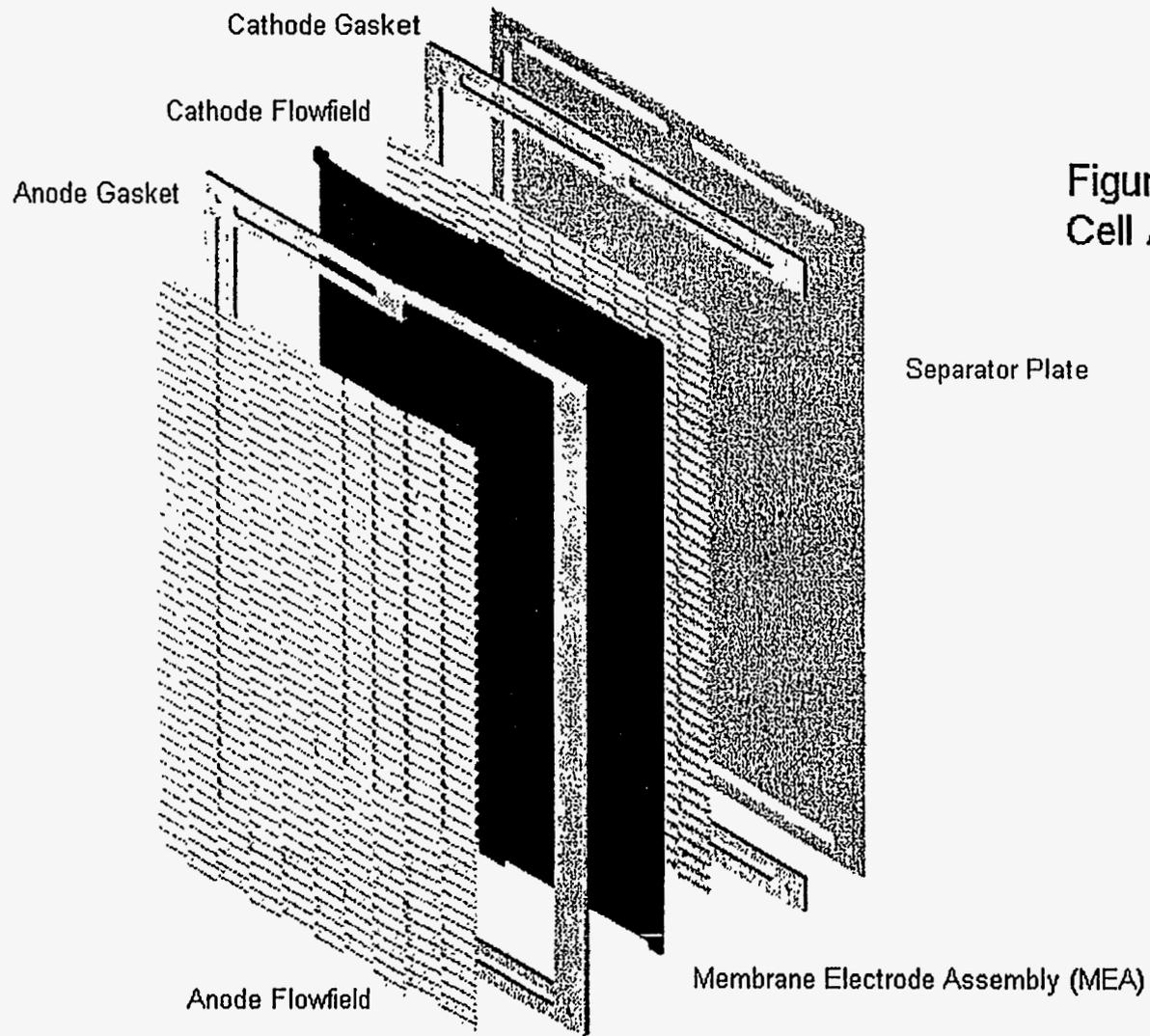
Figure 3: Three-piece Metallic Cell Cell Assembly Schematic
