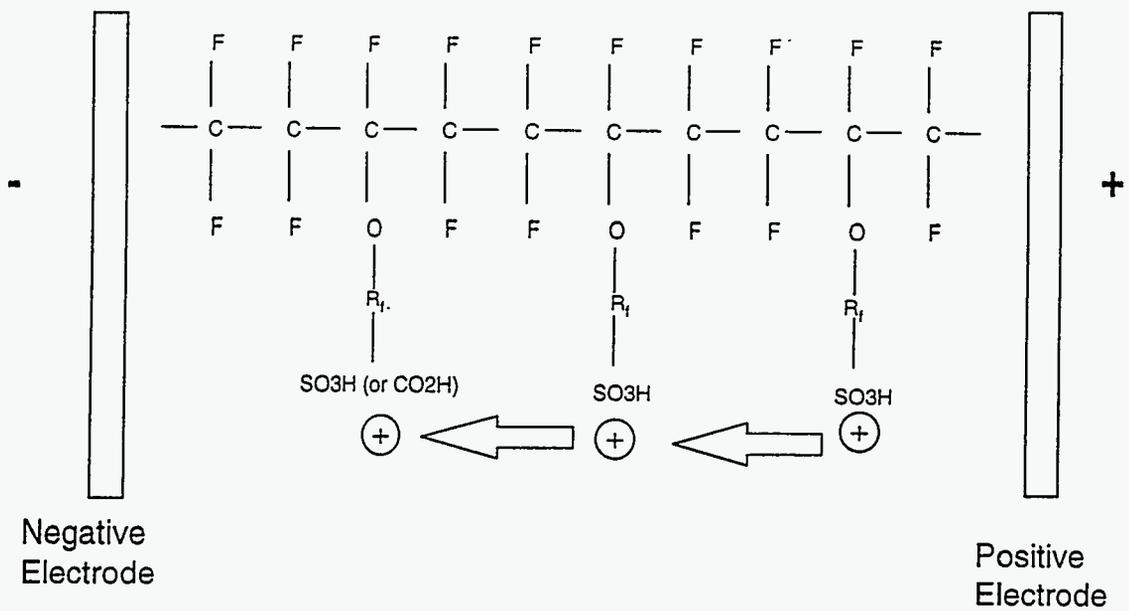
Figure 7 PEM Electrolysis Cell Reactions
