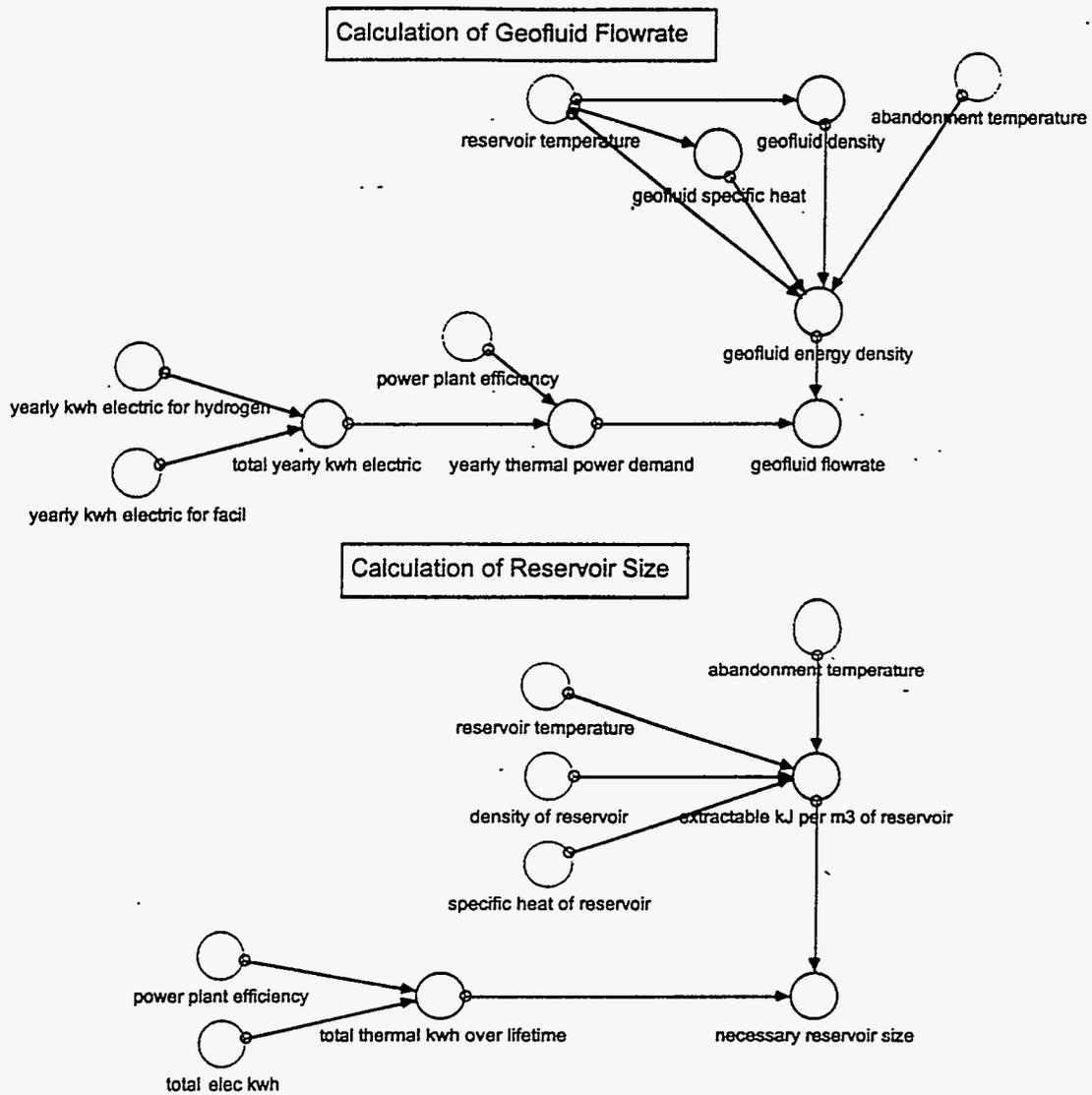
Fig.1. Schematic of the geothermal hydrogen system model. (from Fioravanti (1996)).
