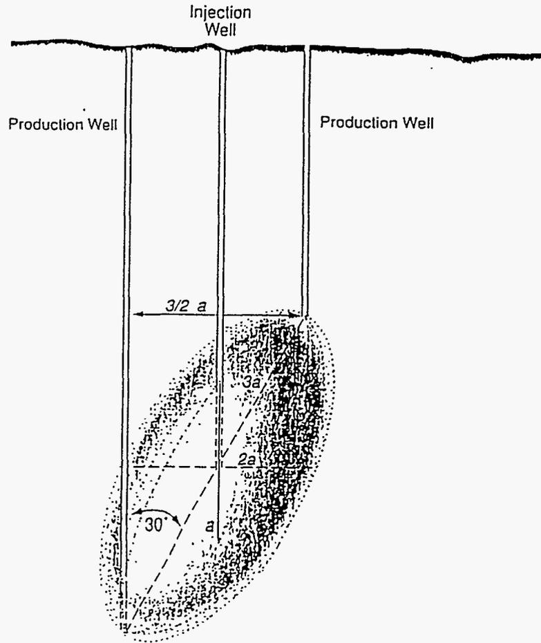
Fig. 5. A conceptual HDR reservoir/wellbore module for a spaceport application, with axis ratios of 3:2:1. The major axis ( $3a$ ), along the direction of the least principle stress, is tilted  $30^\circ$  from the vertical. The injection wellbore is located at the center of the reservoir. Production wells are positioned at each end of the major axis. Circulating fluid flows preferentially along this axis.
