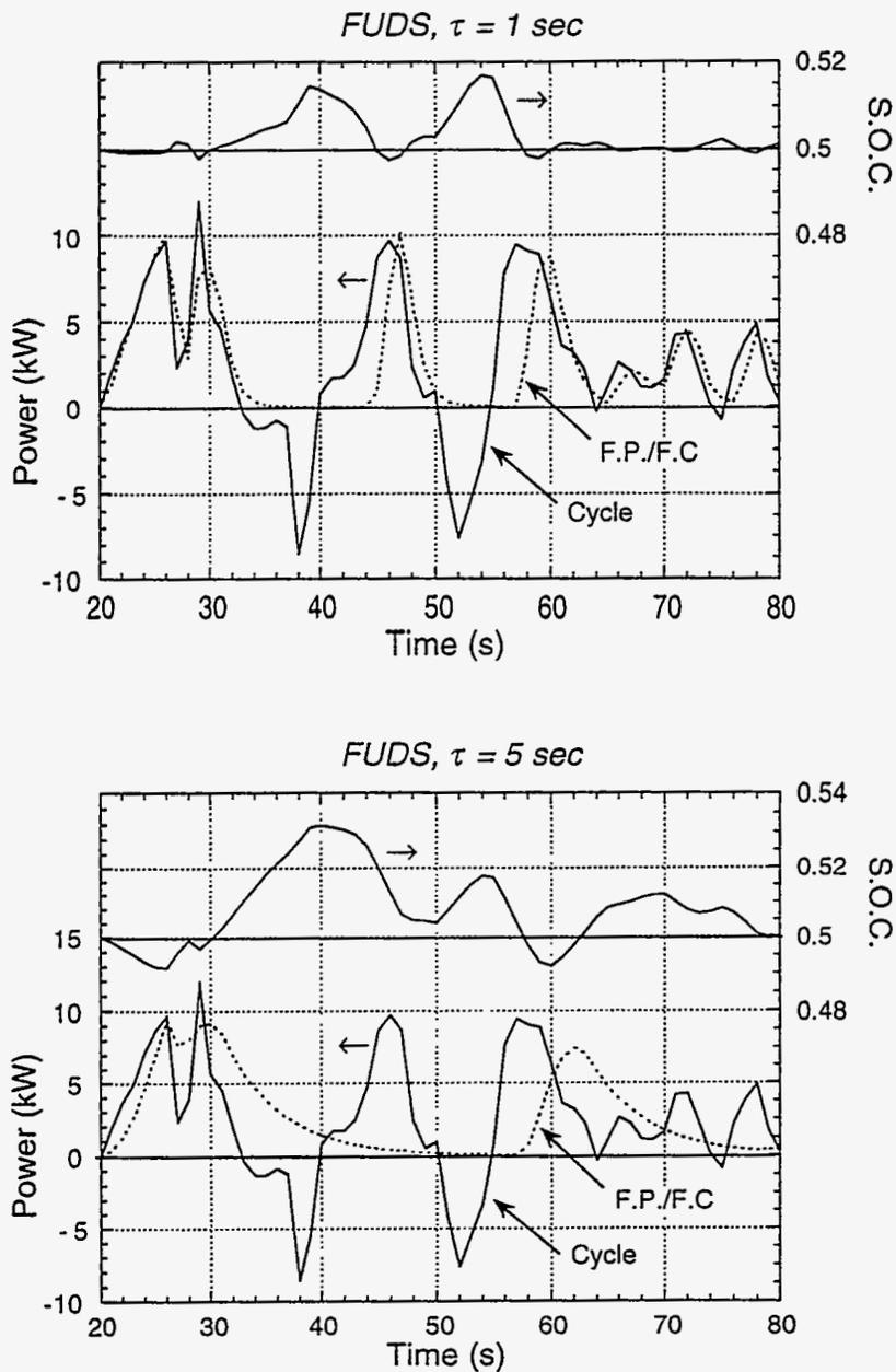
Figure 6. The power provided by the fuel processor/fuel cell - for both 1 and 5 second time constants - as a function of time in response to the power demanded by a portion of the FUDS cycle. The resulting battery fractional state of charge (SOC) is also shown, oscillating about its target value of 50%. Conditions: 1000 kg vehicle mass, 0.36 kWh battery, 1 sec characteristic time for battery recharging, 28.9 kW baseload power, 0.77 motor/controller efficiency.
