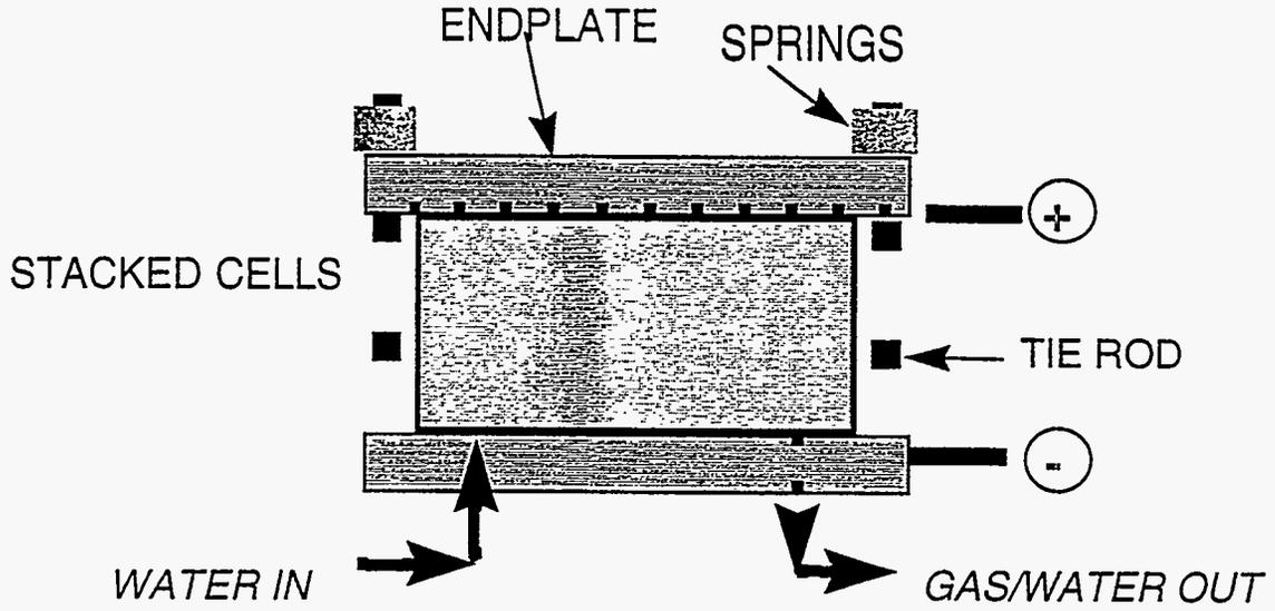
Figure 10 Simplified HOGEN Fluid Schematic
