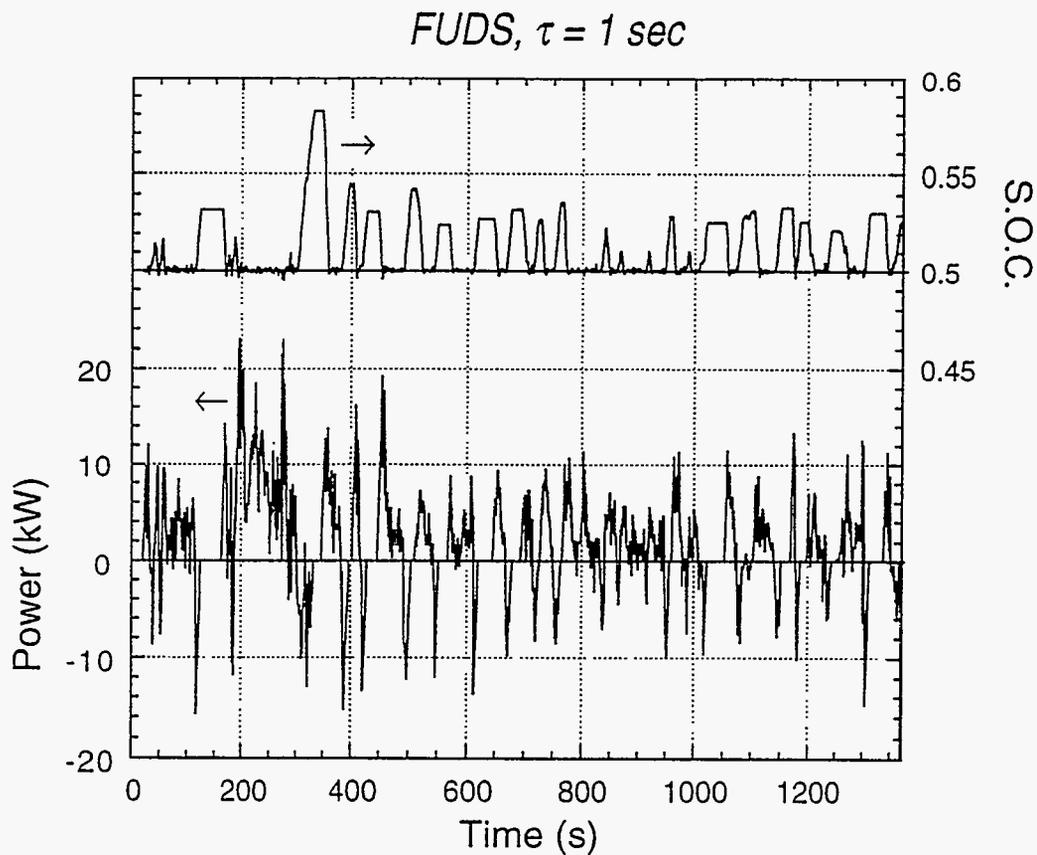
*Figure 5.* The power required of the fuel processor/fuel cell system during the FUDS cycle, and the resulting fractional battery state-of-charge (SOC). Conditions: 1000 kg vehicle mass, 1 sec fuel processor time constant, 0.36 kWh battery, 1 sec characteristic time for battery recharging, 28.9 kW baseload power, 0.77 motor/controller efficiency.
