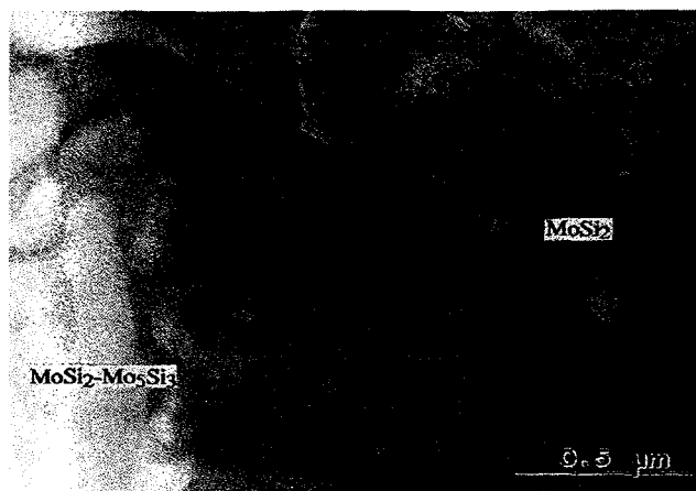
Figure 2: TEM micrograph of as-sprayed MoSi 2 showing the presence of a MoSi 2 -Mo 5 Si 3 eutectic.
