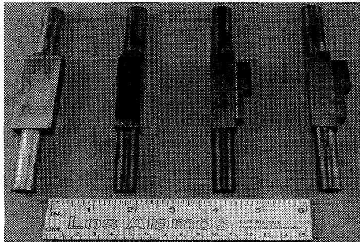
Figure 8. Plasma sprayed beryllium/copper mockups with 5 and 10mm thick individual beryllium tiles used for electron beam high heat flux testing.
