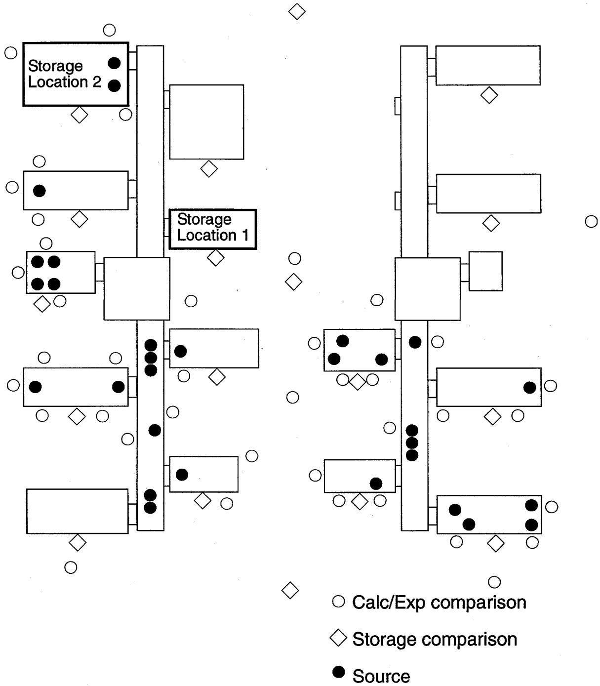
Figure 1. Overhead view of glovebox layout for the calculation/experimental comparison and for the storage comparison.
