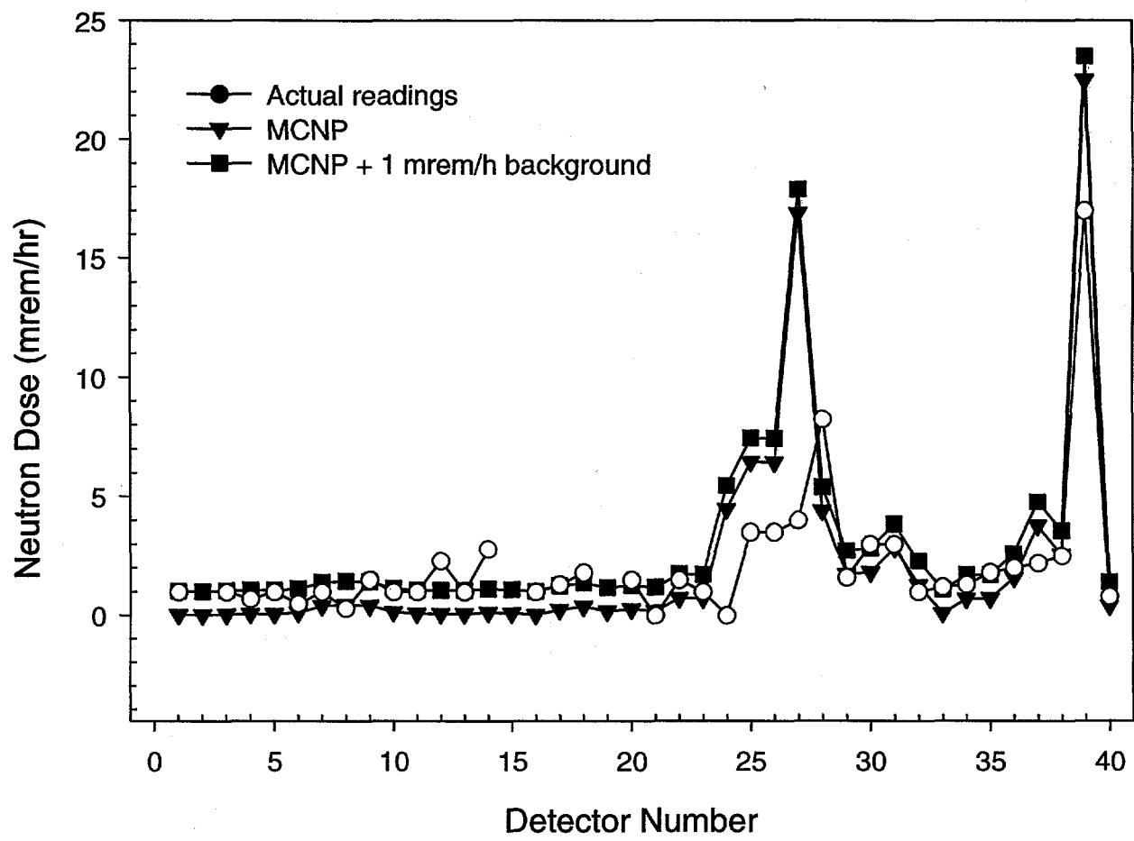
Figure 2. Comparison of measured and calculated neutron dose rates in a room.
