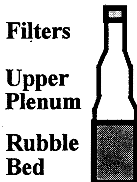
Figure 12. Schematic of the Phebus FPT-4 test configuration.
