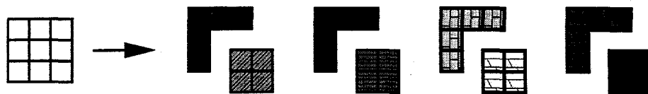
Fig. 8. LLNL's two-step parallelization scheme, where one subset of two processors simulates a single processor in the Full Replication scheme. Each processor subset uses Full Domain Decomposition to represent the whole mesh.
