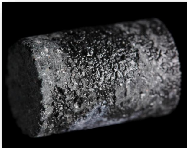
A spent nuclear fuel pellet (about the size of a gummy bear)
