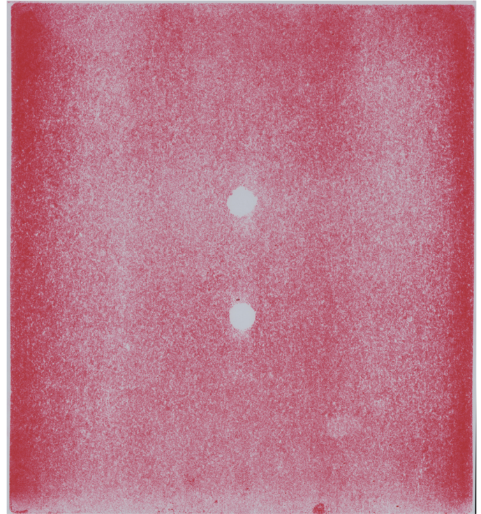
Fig. 2. Pressure-sensitive film, showing the stress distribution on the fracture surface. Higher color intensity indicates higher stress levels and smaller local apertures around the lower borehole compared to the upper one.
