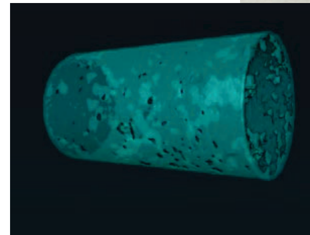
Tomography of NBG-18 sample exposed to molten FLiNaK, 3 bar, 750°C, 336 hours
