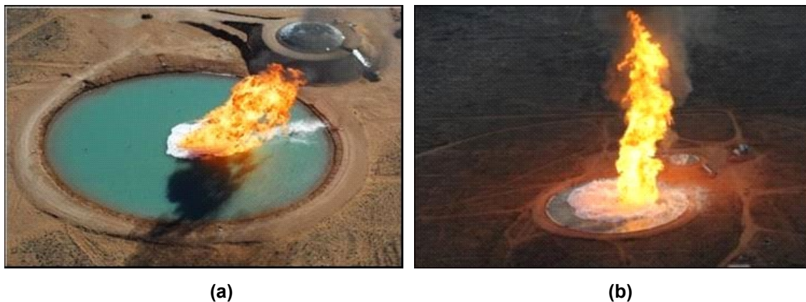
Figure 3-2: Sandia Phoenix 21-m pool fire Test 1 (a) and 56-m pool fire Test 2 (b).
