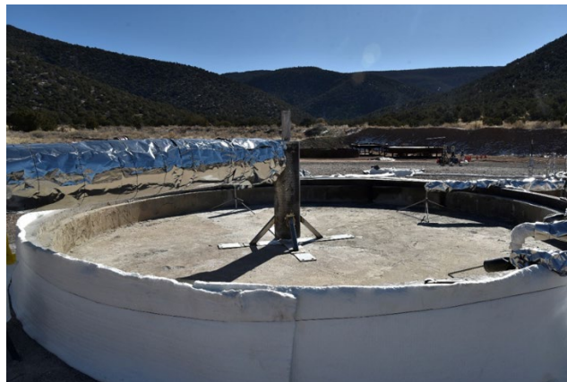
Figure 4-3: Diffuser attached to pipeline for Sandia pool fire experiments.
