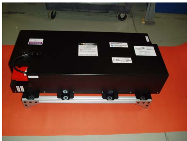
Figure III-60: JCS 344-Volt battery pack
