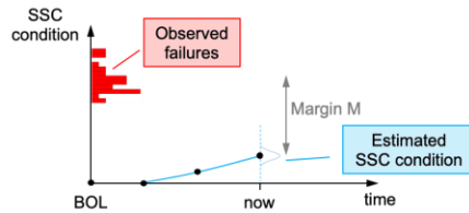
Figure 7. Margin in a condition based maintenance context: evolution of an SSC condition as a function of time and margin definition.
