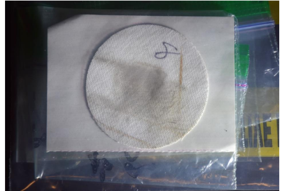
Close-up view of cotton-fiber HP smear, still attached to wax paper backing
