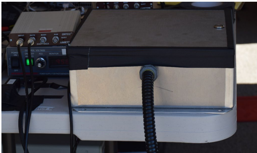
Figure 23. Light-tight box containing the optical fiber and the PMT.
