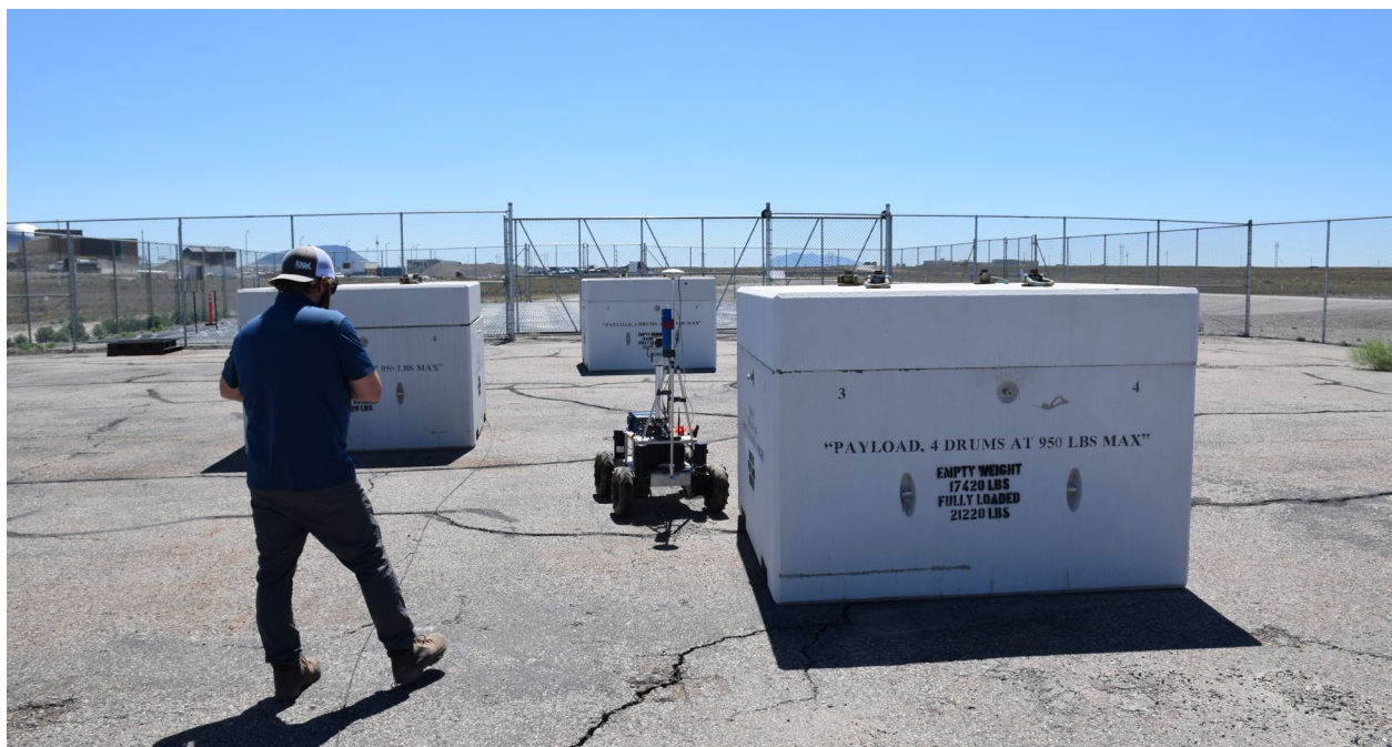
Figure 8. Remote-controlled rover system equipped with a sodium iodide gamma-ray detector.
