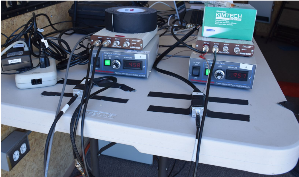
Figure 5. Data acquisition system inside the trailer.
