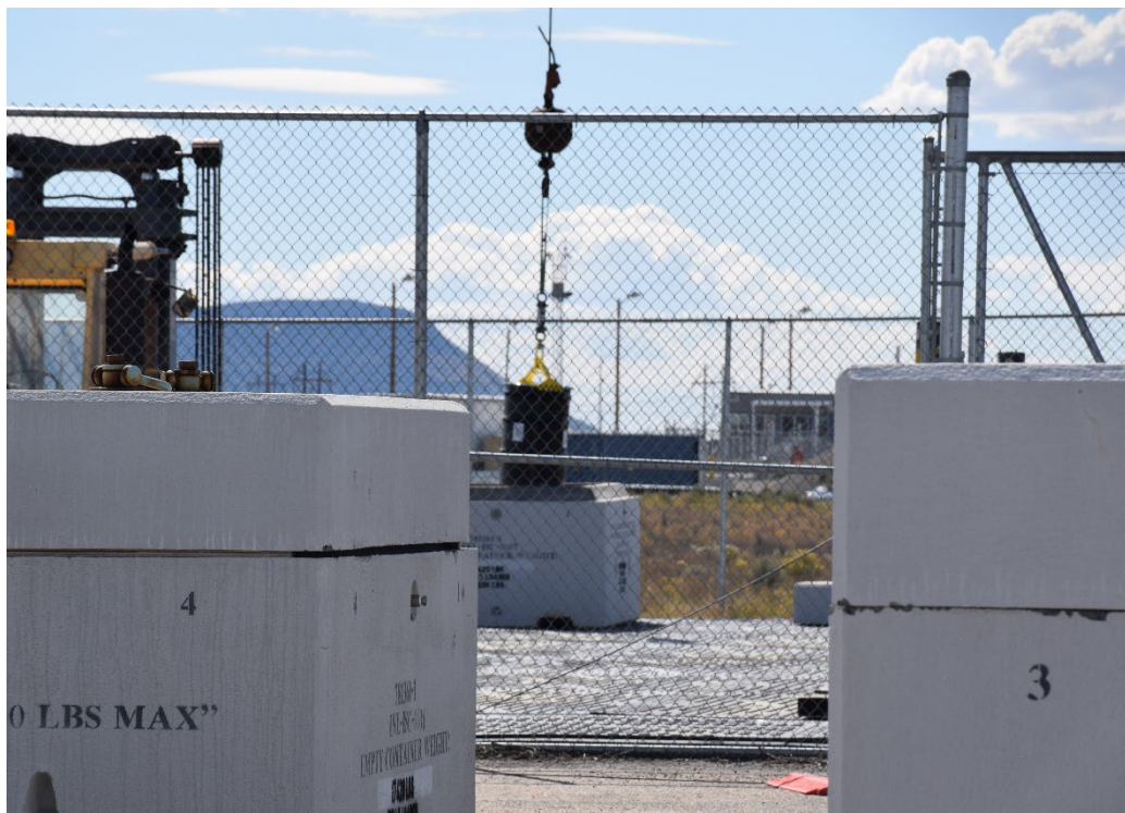
Figure 24. Lowering of the 50 gallon drum into the fourth position of ISC-007.
