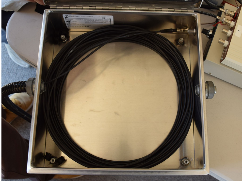
Figure 22. Optical fiber coiled inside a light-tight box to prevent unwanted photons from light sources in the trailer.
