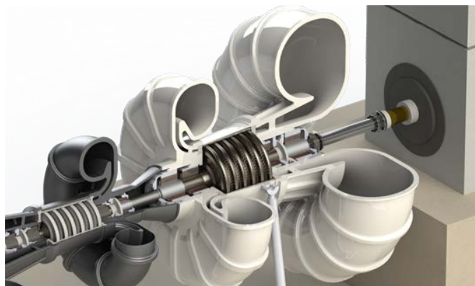
Figure 44. Schematic design of the Brayton Energy reversible turbomachinery for PTES from Brayton's ARPA-E DAYS project. The turbomachine requires large, thick-walled volutes to deliver and receive the flow to the heat sources, such as the NLR FB. This 50-MW e machine was designed for 5-bar inlet pressure and 15-bar exit pressure.
