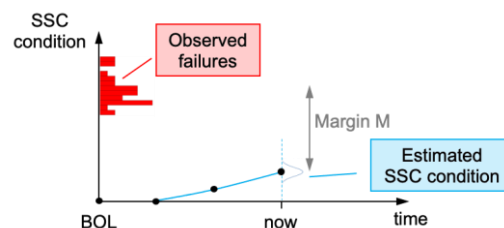
Figure 6. Margin in a condition-based maintenance context: evolution of an SSC condition as a function of time and margin definition.
