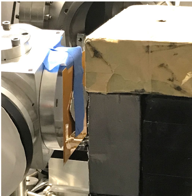
Figure 22 Beam output window with Indium foil and radiochromatic film.
