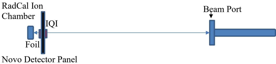
Figure 64 Diagram of setup with NOVO panel and components.
