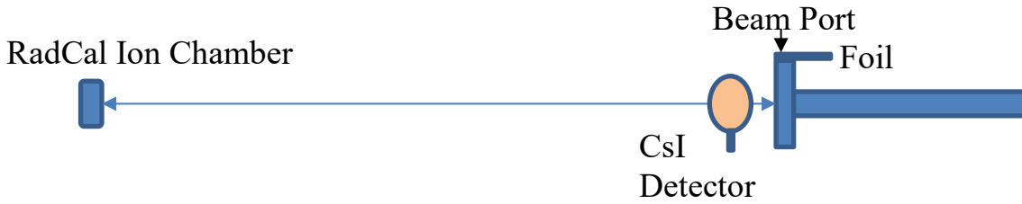
Figure 24 Diagram of setup and components with Thomson photons. Measurement 1.7
