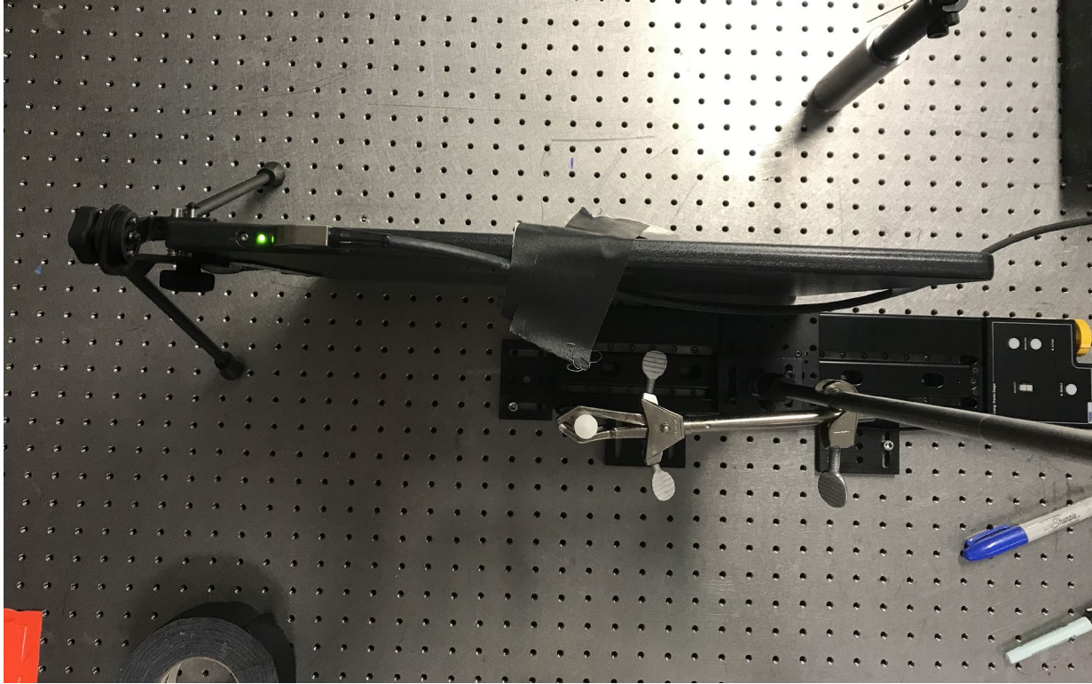
Figure 34 Top view of the NOVO detector and ion chamber.
