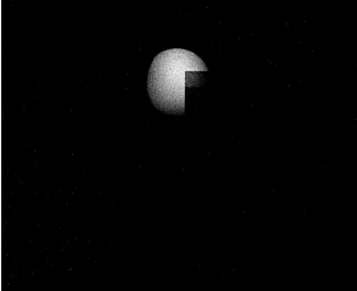
Figure 58 Thomson Photon Exposure:175 seconds (average of 5) of step wedge. Image centered on first step.
