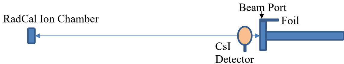
Figure 26 Diagram of setup and components with Thomson photons. Measurement 1.8
