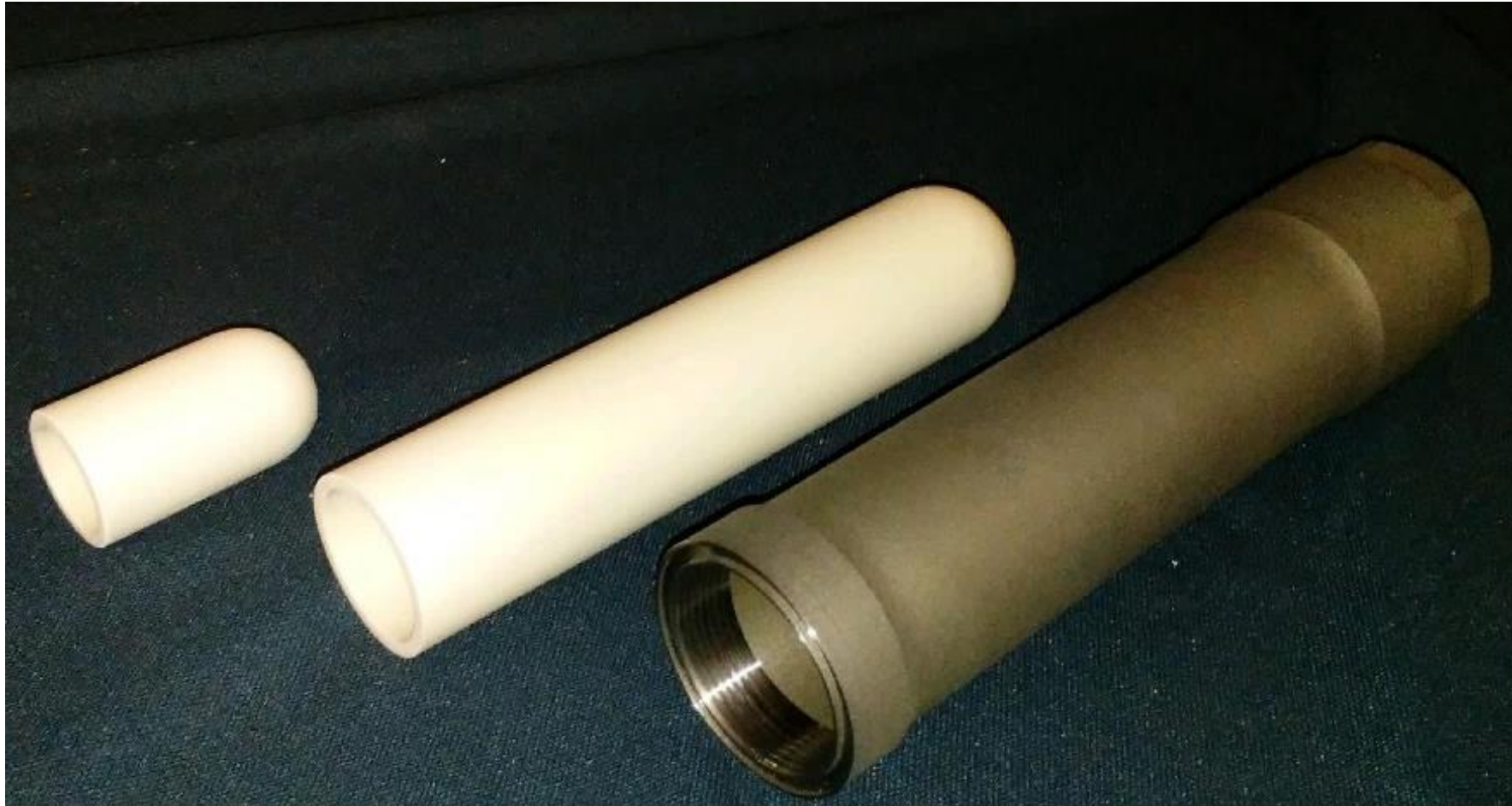
'SETH' test capsule with crucible liners
