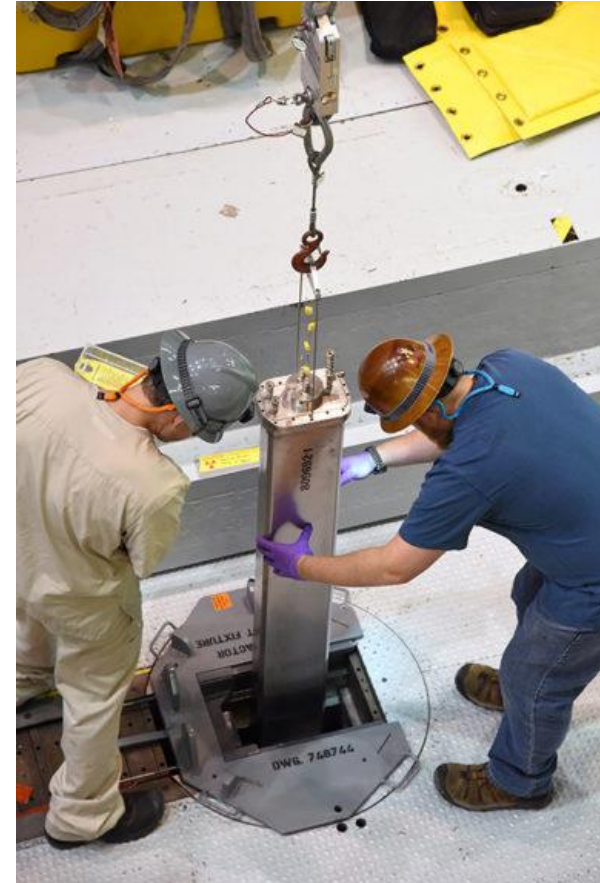
Insertion of a test rig into the TREAT reactor
